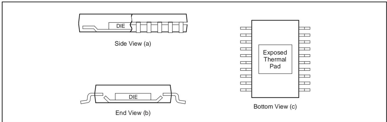
**Figure 9. SO-20 Package Example of Thermally Enhanced PowerPAD**
