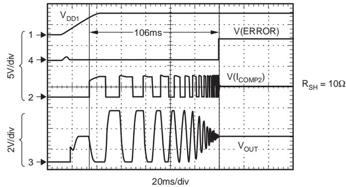
a) Demagnetization cycle on power-up. With power-up, the  $V_{OUT}$  across the compensation coil centers around half the supply and then starts the cycle after the 4V threshold is exceeded. The ERROR flag resets to H after the cycle is completed.
