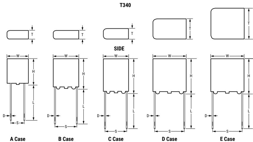
F case size is the same as D, but with 0.200" (5.0 mm) lead spacing. Specify T340F when ordering this spacing.
