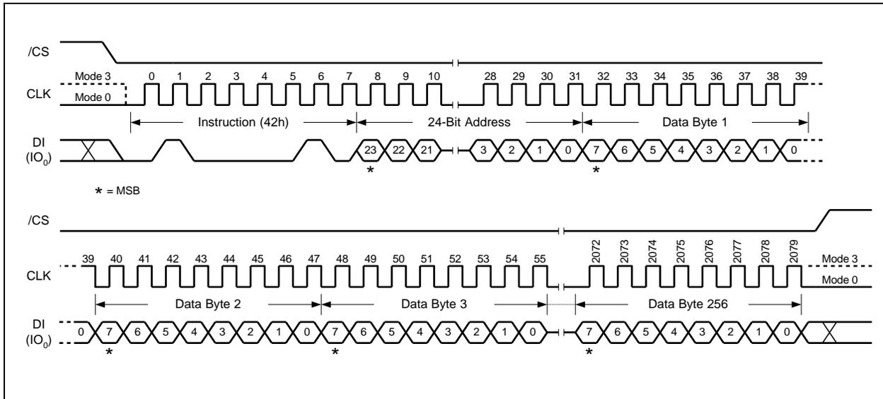
Figure 46. Program Security Registers Instruction (SPI Mode only)
