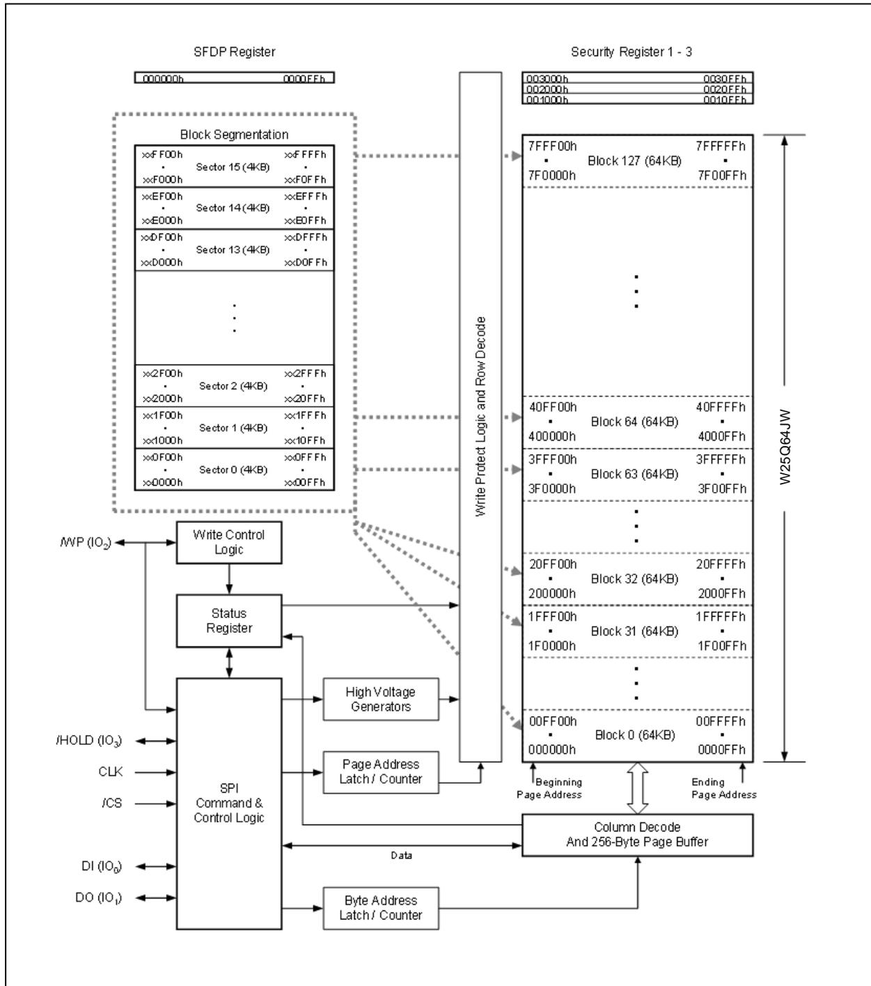
Figure 2. W25Q64JW Serial Flash Memory Block Diagram
