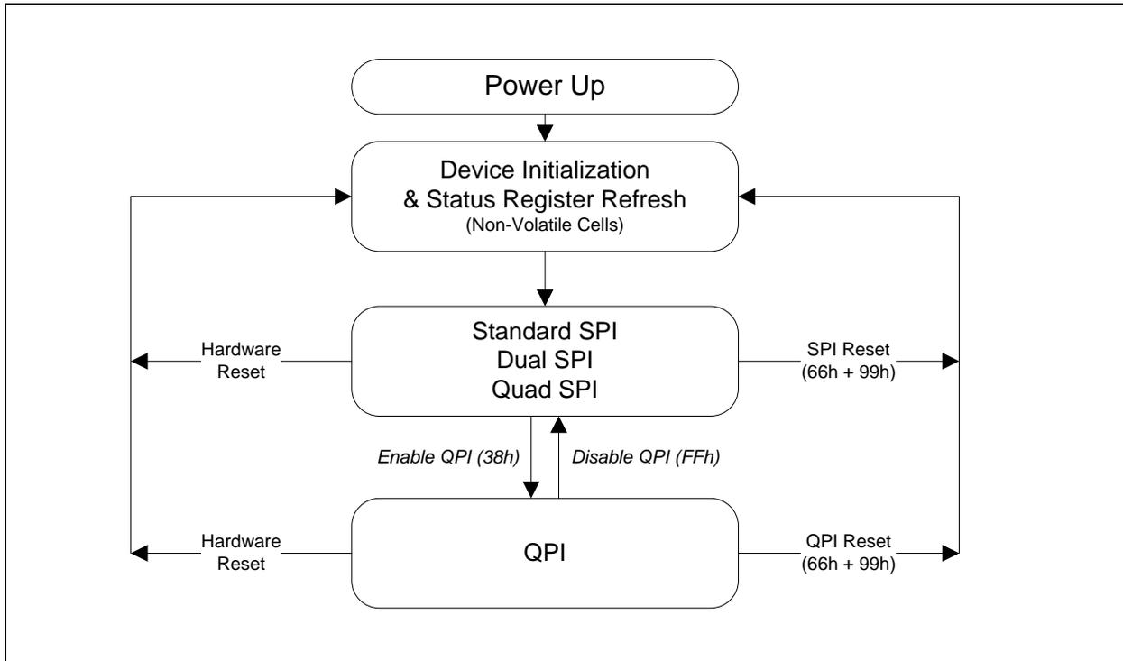
Figure 3. W25Q64JW Serial Flash Memory Operation Diagram
