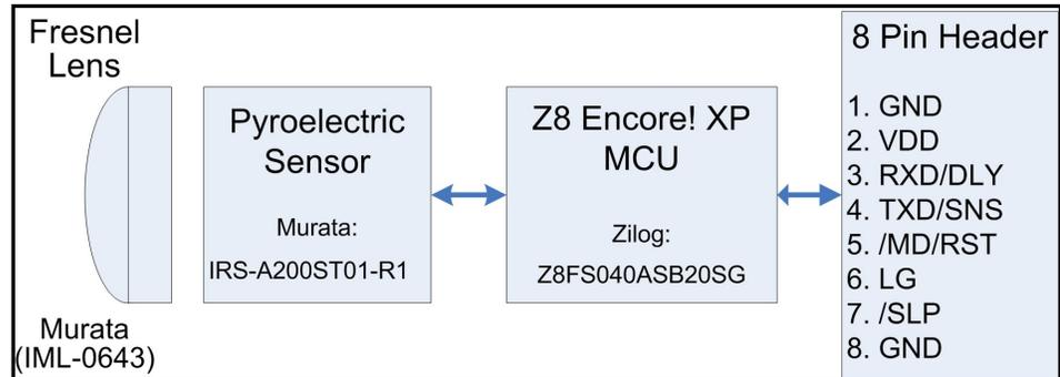
The ePIR Motion Detection Zdots SBC uses a Fresnel lens to break up the radiated IR energy into multiple concentrated images. These images are refracted on to the element of the PIR sensor which generates a signal based on the change in energy. The signal is fed directly to the Z8 Encore! XP MCU where it is analyzed by the motion detection algorithms to determine if it is from a valid source.
