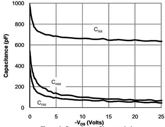
**Figure 8: Capacitance Characteristics**
