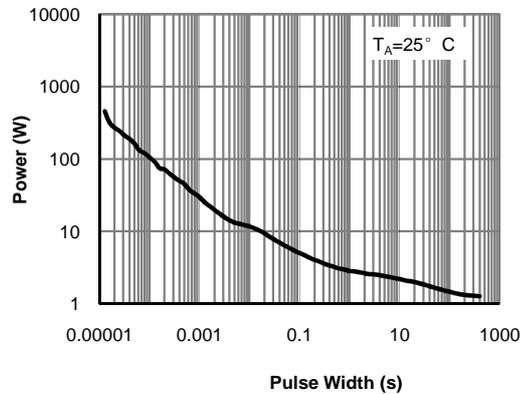
**Figure 10: Single Pulse Power Rating Junction-to-Ambient (Note F)**
