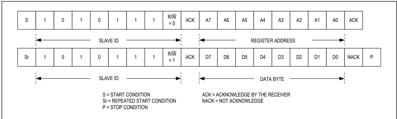
Figure 10. Reading One Byte of Data from MAX30102
