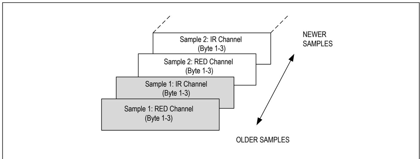
Figure 2. Graphical Representation of the FIFO Data Register. It shows IR and Red in SpO<sub>2</sub> Mode.
