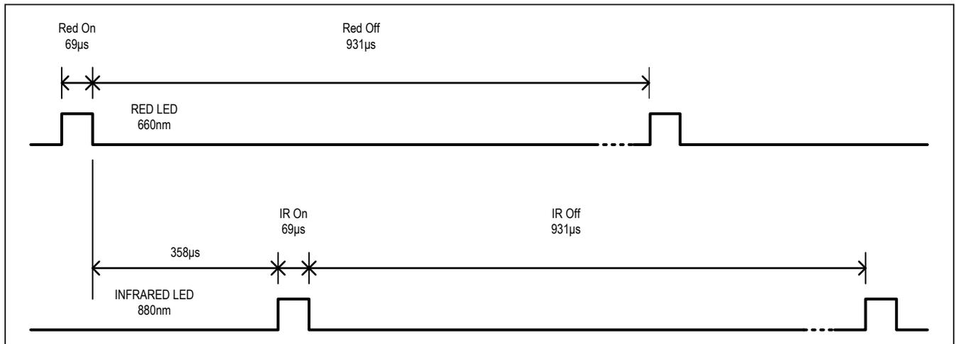
Figure 3. Channel Slot Timing for the SpO<sub>2</sub> Mode with a 1kHz Sample Rate
