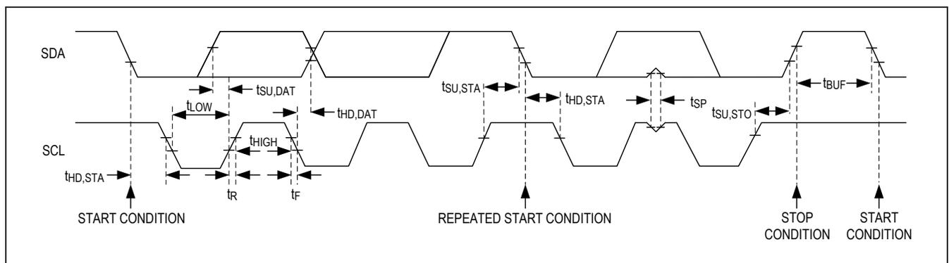
Figure 1. I<sup>2</sup>C-Compatible Interface Timing Diagram
