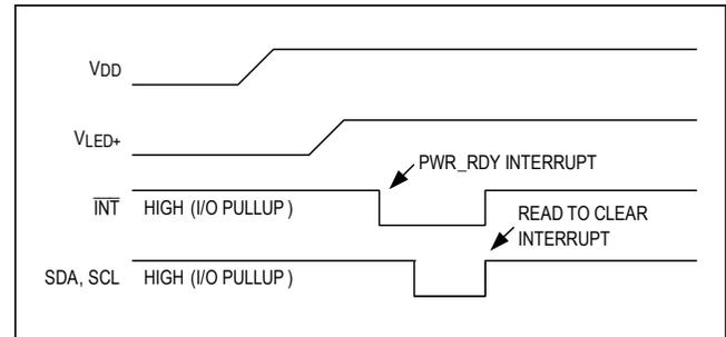
Figure 6. Power-Up Sequence of the Power Supply Rails
