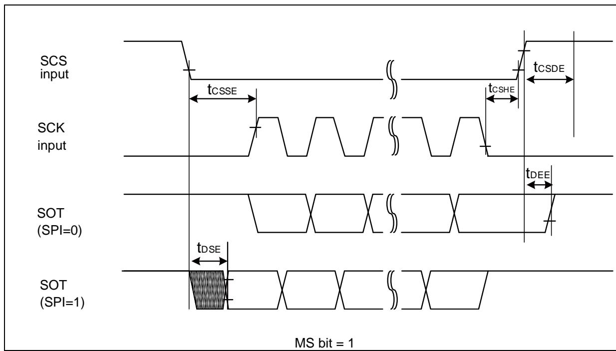
**When Using Synchronous Serial Chip Select (SCINV = 0, CSLVL = 0)**
