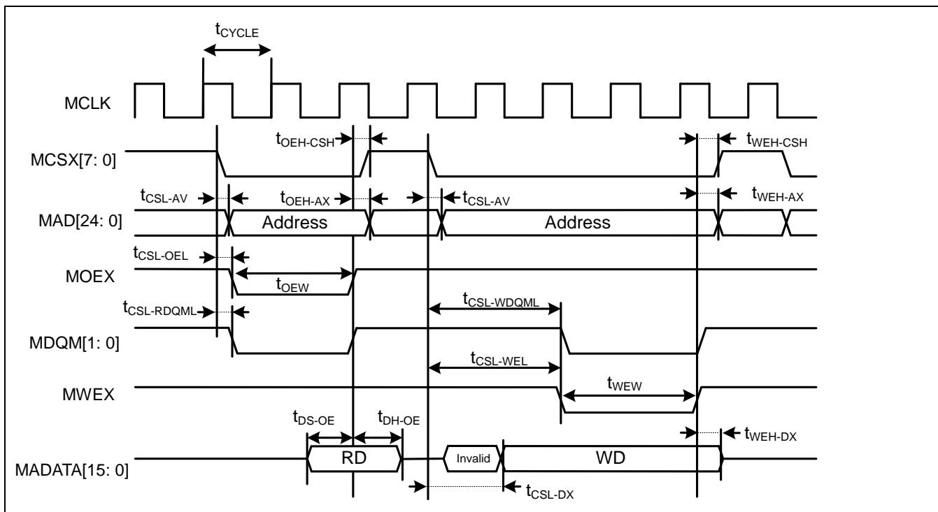
**Separate Bus Access Synchronous SRAM Mode**
