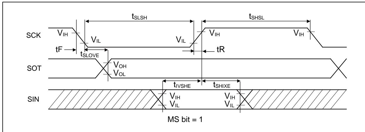
**High-Speed Synchronous Serial (SPI = 0, SCINV = 1)**
