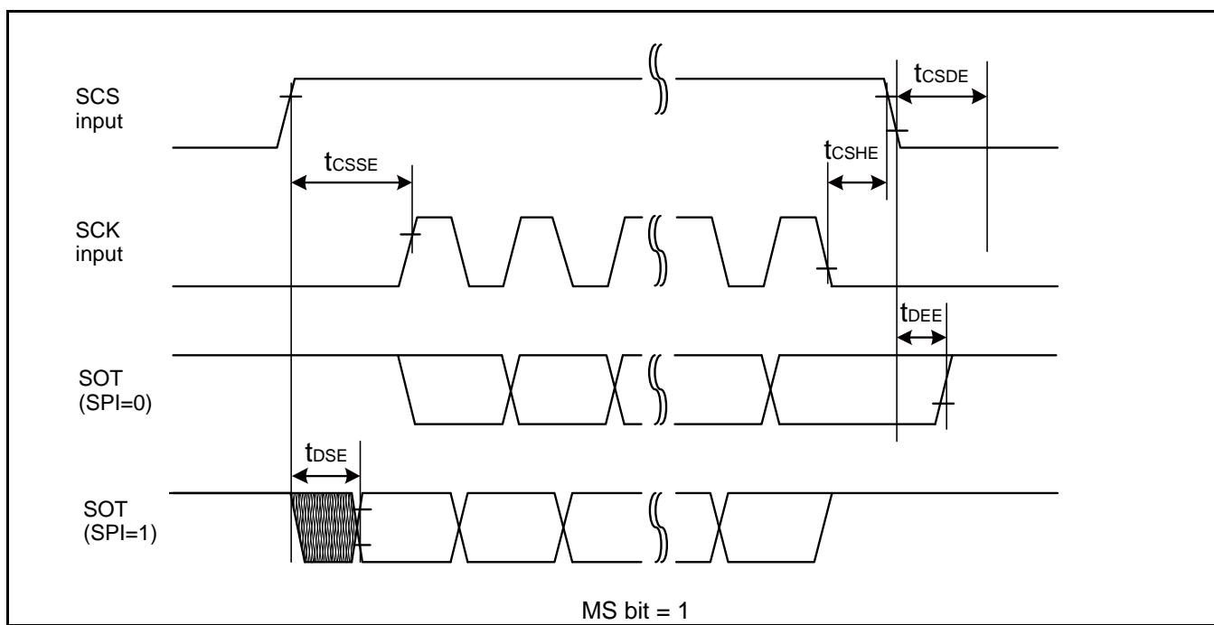
**External clock (EXT = 1): When in Asynchronous Mode Only**
