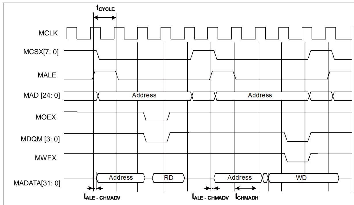
**Multiplexed Bus Access Synchronous SRAM Mode**
