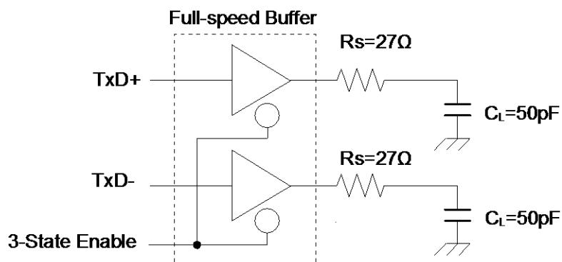
\*6: USB Full-speed connection is performed via twisted-pair cable shield with  $90\ \Omega \pm 15\%$  characteristic impedance (differential mode).
