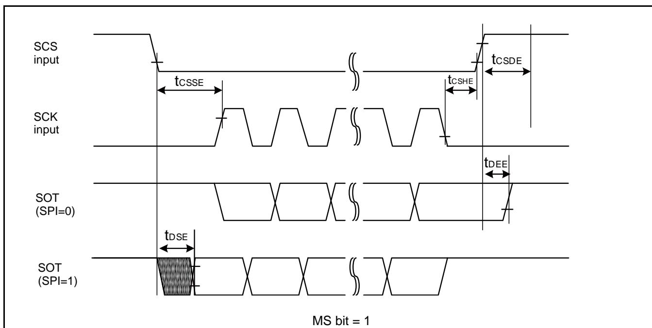
**When Using High-Speed Synchronous Serial Chip Select (SCINV = 0, CSLVL = 0)**
