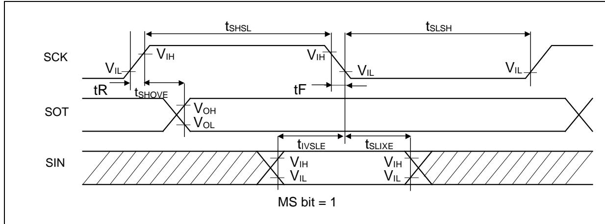
**High-Speed Synchronous Serial (SPI = 1, SCINV = 0)**
