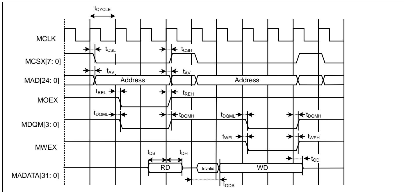
**Multiplexed Bus Access Asynchronous SRAM Mode**
