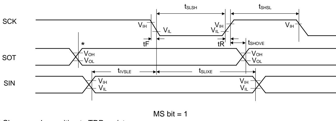
**Synchronous Serial (SPI = 1, SCINV = 1)**
