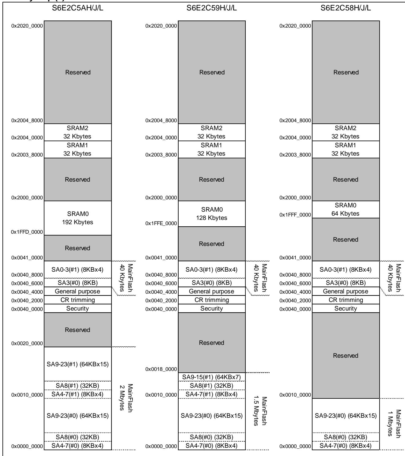
\* See S6E2CC/S6E2C5/S6E2C4/S6E2C3/S6E2C2/S6E2C1 Series Flash Programming Manual to confirm the detail of flash Memory.
