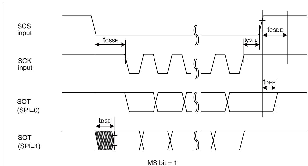
**When Using Synchronous Serial Chip Select (SCINV = 1, CSLVL = 1)**
