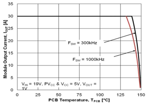
Figure 5. Safe Operating Area with 19  $V_{IN}$
