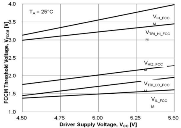
Figure 19. FCCM Threshold vs. Driver Supply Voltage
