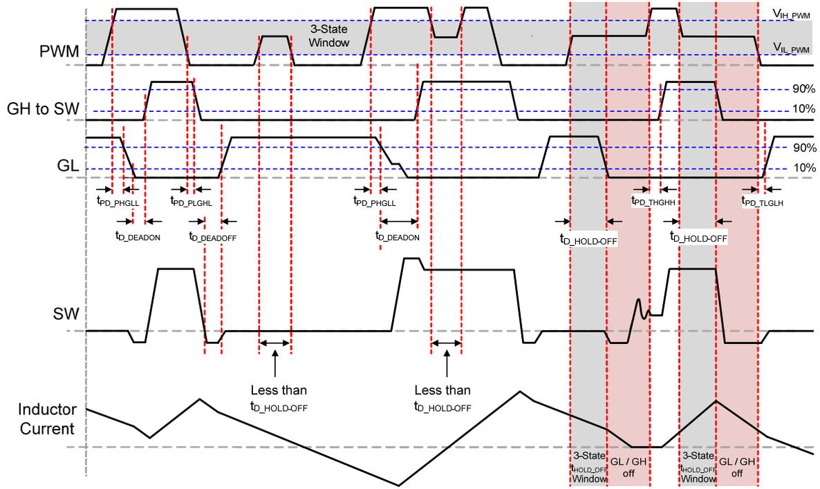
**Figure 29. PWM 3-State Timing Diagram (FCCM held HIGH)**
