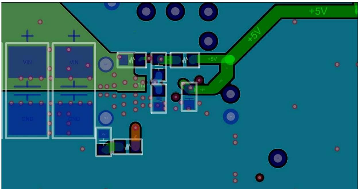
Figure 33. Single-Phase Board Layout Example – Bottom View (Mirrored)
