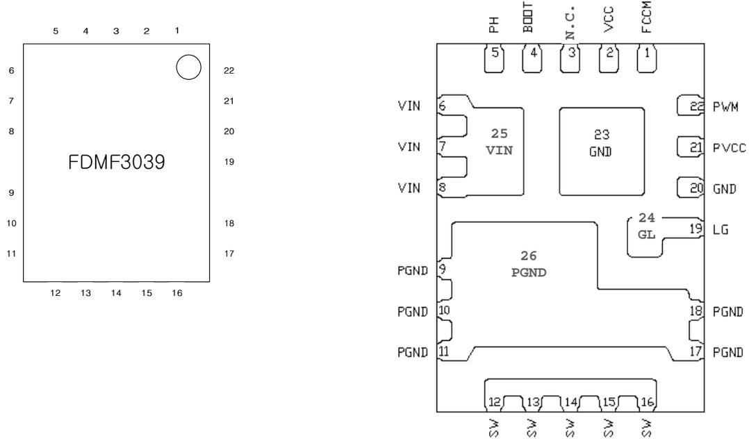
Figure 3. Pin Configuration - Top View and Transparent View
