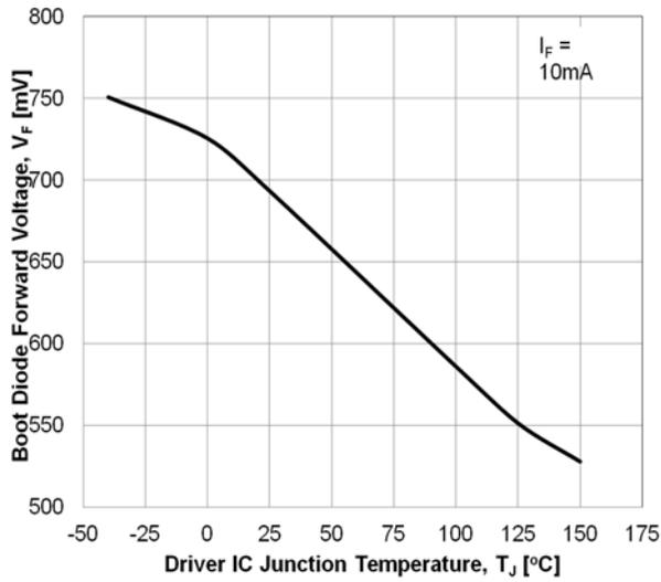
Figure 22. Boot Diode Forward Voltage vs. Temperature
