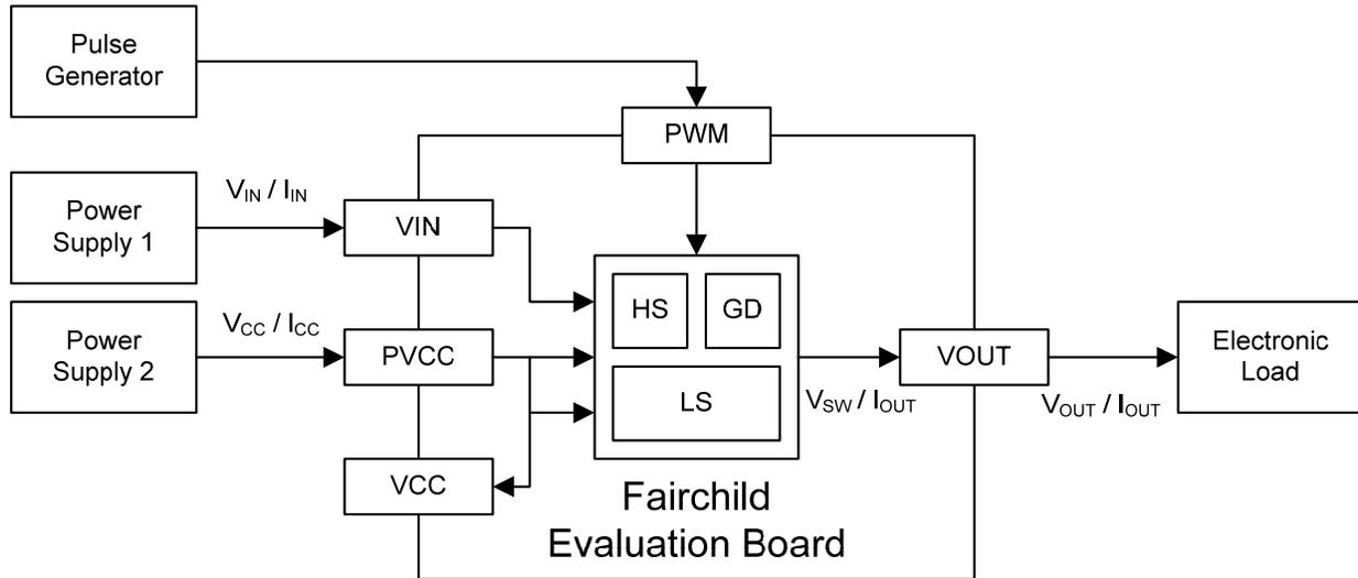
Figure 31. Power Loss and Efficiency Measurement Diagram
