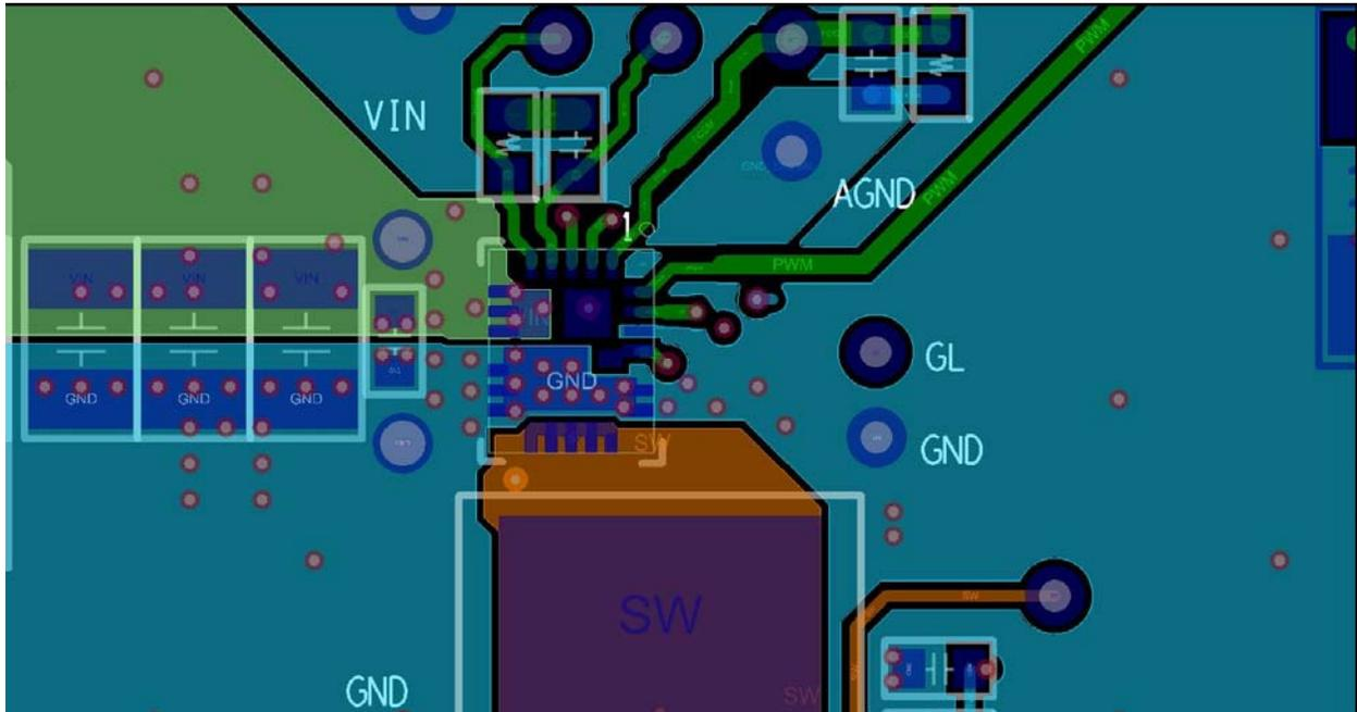
Figure 32. Single-Phase Board Layout Example – Top View
