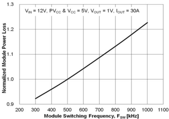
Figure 8. Power Loss vs. Switching Frequency
