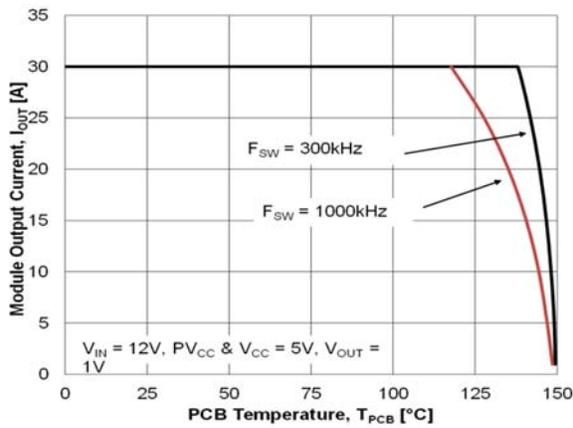
Figure 4. Safe Operating Area with 12  $V_{IN}$
