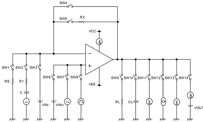
Figure 49. Test circuit 2 (one channel only)
