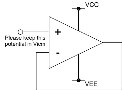
Figure 54. Unused circuit example
