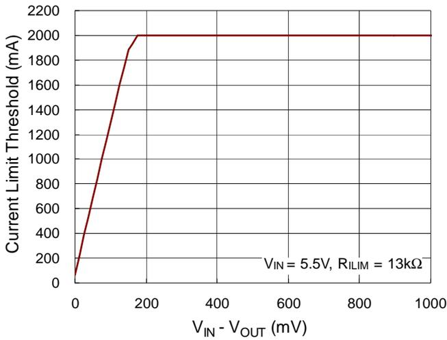
Current Limit Threshold vs. ( $V_{IN} - V_{OUT}$ )
