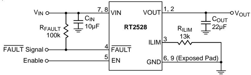
Note :  $R_{ILIM} = 13k\Omega$  for 2A Power Switch Operation
