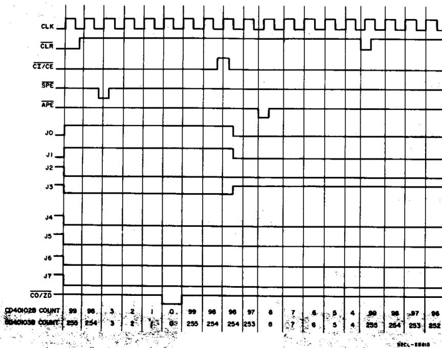
Fig. 15 - Timing diagram for CD40102B and CD40103B.
