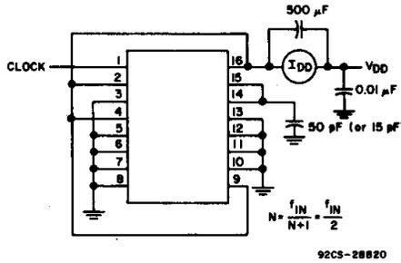
Fig. 17 - Dynamic power dissipation test circuit (÷2 mode).
