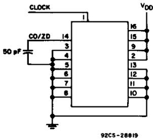
Fig. 16 - Maximum clock frequency test circuit.
