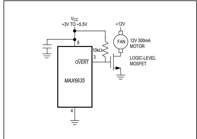
Figure 11. Fan Controller
