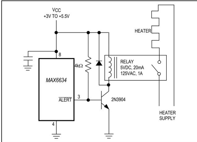
Figure 10. Simple Thermostat
