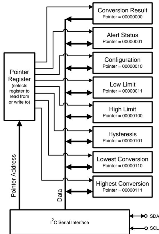
Figure 21. Register Structure
