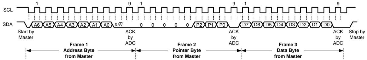
**Figure 30. Typical Write to a 1-Byte ADC Register**
