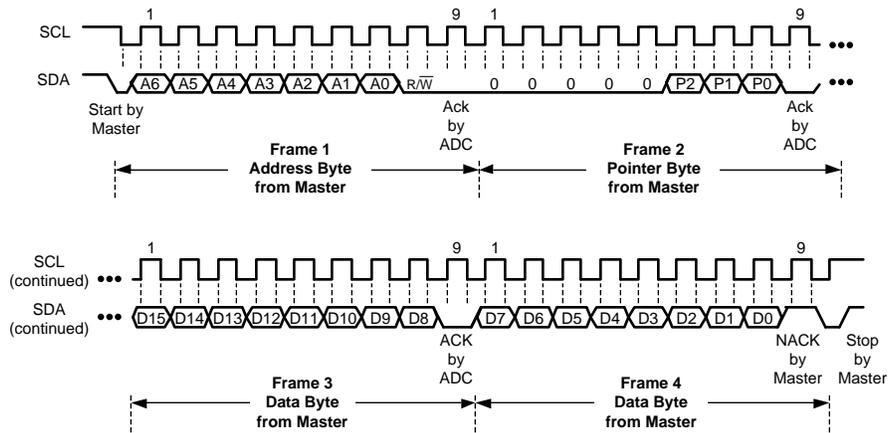
**Figure 31. Typical Write to a 2-Byte ADC Register**
