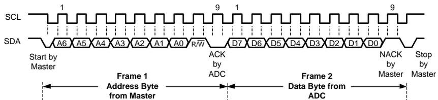
Figure 28. Typical Read from a 1-Byte ADC Register with Preset Pointer
