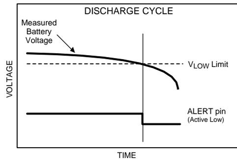
Figure 37. Discharge Cycle
