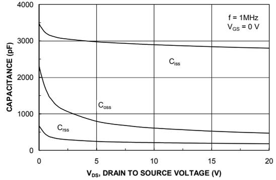
Figure 8. Capacitance Characteristics.
