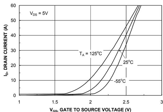
Figure 5. Transfer Characteristics.
