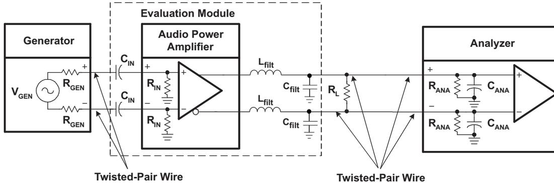
Figure 31. Differential Input, BTL Output Measurement Circuit
