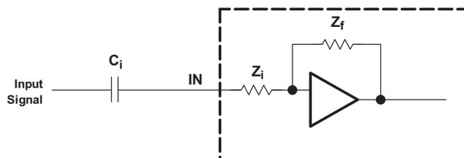
The  $-3$ -dB frequency can be calculated using [Equation 1](#). Use the  $Z_i$  values given in [Table 2](#).
