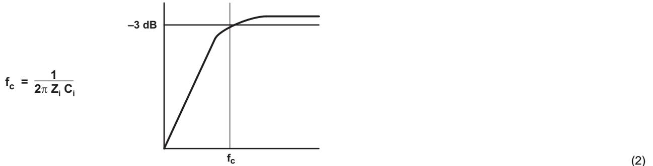
The value of C<sub>i</sub> is important, as it directly affects the bass (low-frequency) performance of the circuit. Consider the example where Z<sub>i</sub> is 20 kΩ and the specification calls for a flat bass response down to 20 Hz. Equation 2 is reconfigured as Equation 3.
