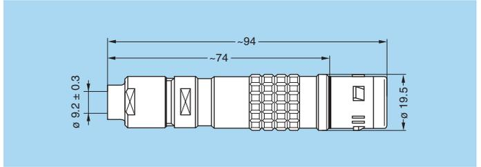
**FXW** Fixed plug, round flange (4 holes mounting), without collet
