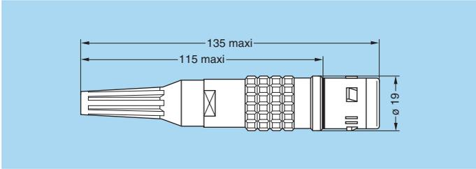
**FUW** Straight plug, cable collet adapter, long shell, nut for fitting a bend relief with cap
