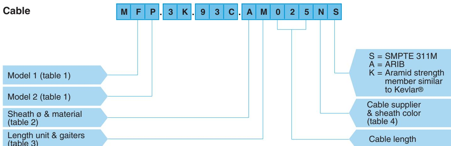
**MFP.3K.93C.AM025NS** = 1 FUW plug and 1 PUW socket (key W), 3K.93C series, on a SMPTE 311M screened cable, 25 m length, sheath ø 9.2 mm, black RAL 9005 jacket color, with GMF/GMP bend relief with cap.
