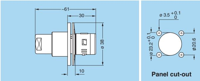
**FMW** Fixed plug, round flange (4 holes mounting), cable adapter, with bend relief
