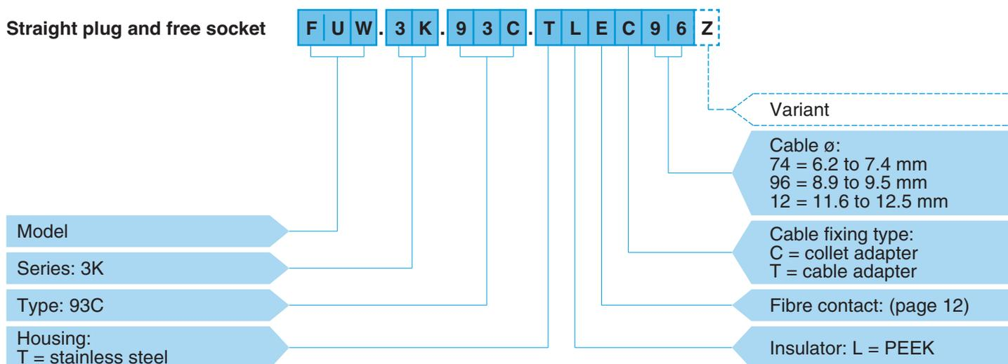
**FUW.3K.93C.TLEC96Z** = Straight plug with keys (W), 3K series, mixed type to accept 2 F2 type fibre optic contacts, 2 power and 2 signal electrical contacts, stainless steel housing, PEEK insulator, female crimp signal contacts, cable fixing type T for 9.2 mm diameter cable, and nut for fitting a bend relief.
