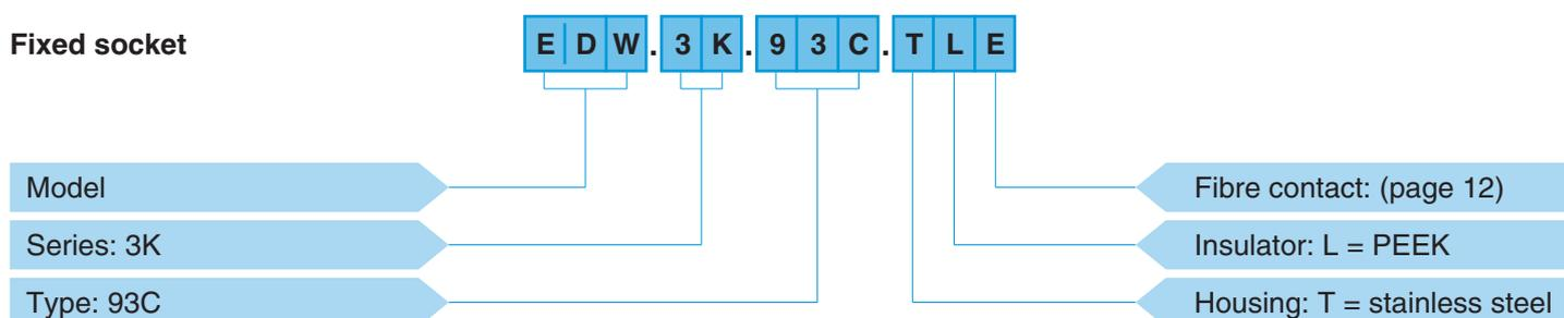
**EDW.3K.93C.TLE** = Fixed socket with rear square flange, keys (W), 3K series, mixed type to accept 2 F2 type fibre optic contacts, 2 power and 2 signal electrical contacts, stainless steel housing, PEEK insulator, male crimp signal contacts.
