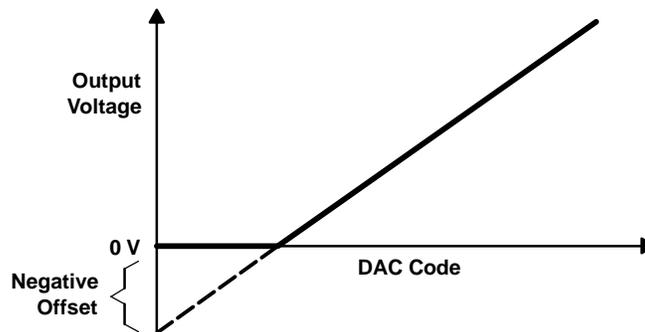
**Figure 15. Effect of Negative Offset (Single Supply)**
