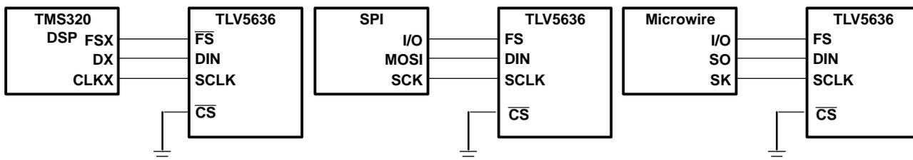
Figure 14. Three Wire Interface
