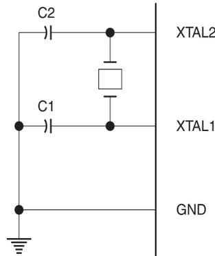
Note: C1, C2 = 30 pF  $\pm$  10 pF for Crystals
