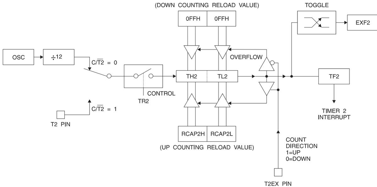
Figure 8-4. Timer 2 in Baud Rate Generator Mode
