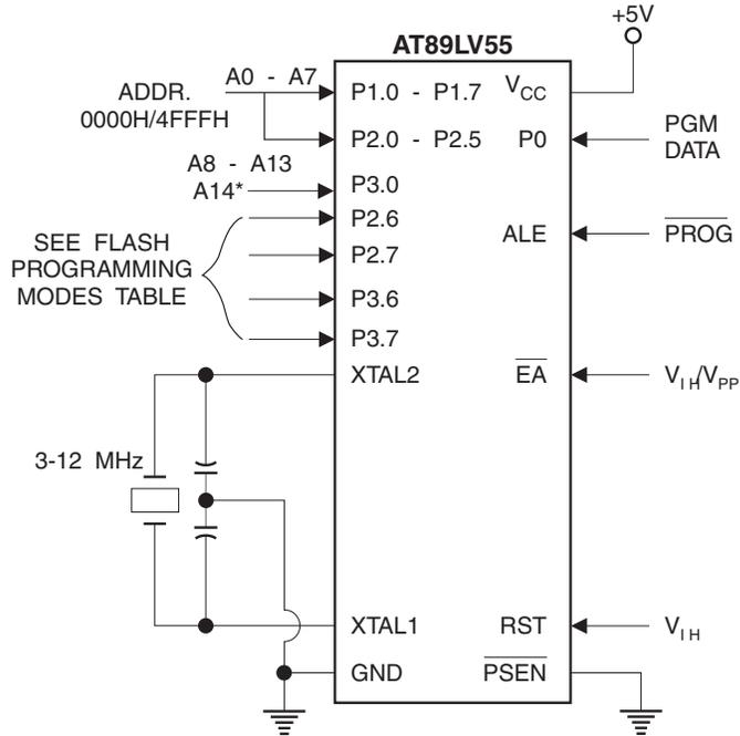
\*Programming address line A14 (P3.0) is not the same as the external memory address line A14 (P2.6)
