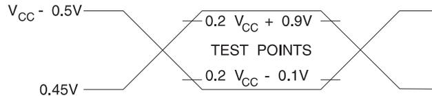
Note: 1. AC Inputs during testing are driven at 2.4V for a logic "1" and 0.45V for a logic "0". Timing measurements are made at 2.0V for a logic "1" and 0.8V for a logic "0".
