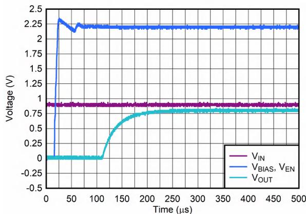
Figure 6-15. Start-Up With  $V_{IN}$  Before  $V_{BIAS}$  and  $V_{EN}$
