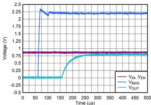
Figure 6-17. Start-Up With  $V_{IN}$  and  $V_{EN}$  Before  $V_{BIAS}$
