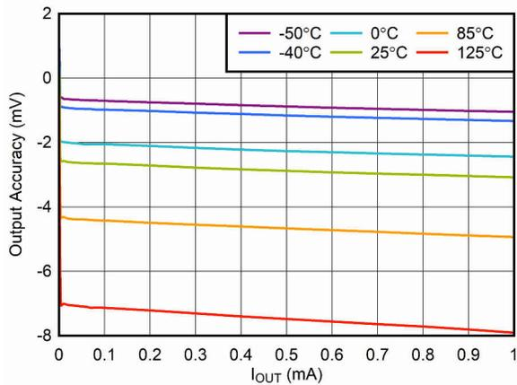
Figure 6-3. Output Voltage Accuracy vs  $I_{\text{OUT}}$
