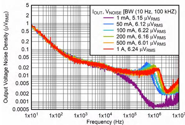
Figure 6-27. Output Noise vs Frequency and  $I_{OUT}$
