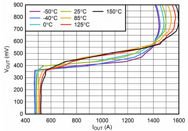
Figure 6-10.  $V_{\text{OUT}}$  Foldback Current Limit vs Output Current
