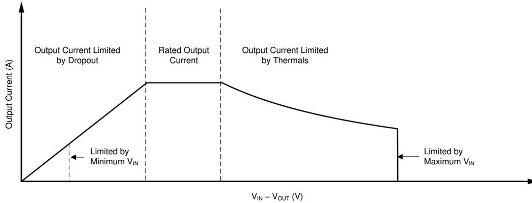
Figure 8-3. Continuous Operation Diagram With Description of Regions
