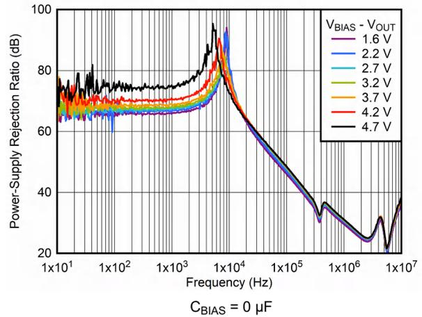
Figure 6-26. PSRR vs Frequency and  $V_{BIAS} - V_{OUT}$
