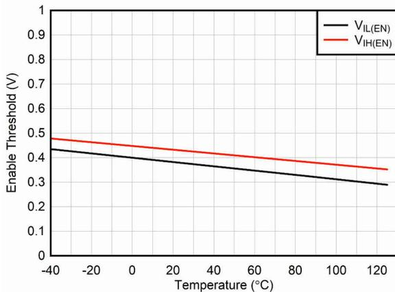
Figure 6-11. Enable Threshold vs Temperature
