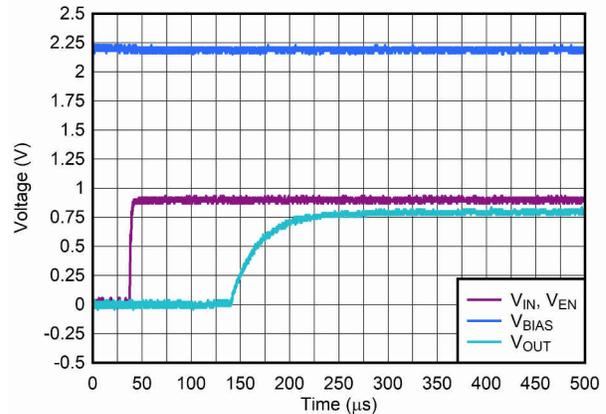
Figure 6-14. Start-Up With  $V_{BIAS}$  Before  $V_{IN}$
