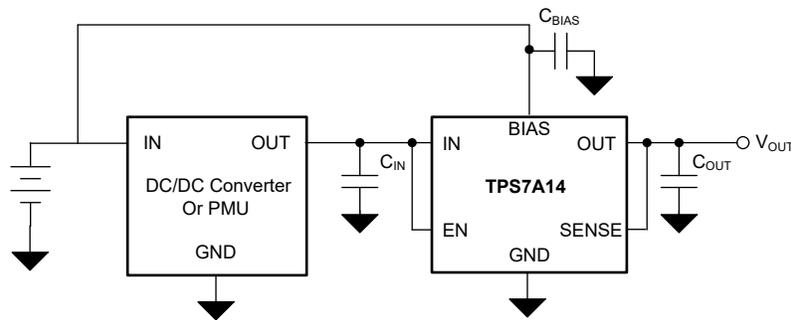
Figure 8-4. High-Efficiency Supply From a Rechargeable Battery
