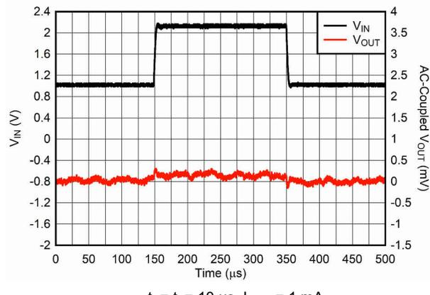
Figure 6-18. Line Transient From 1 V to 2.2 V
