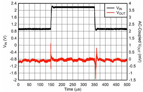
$t_r = t_f = 10\text{ }\mu\text{s}$ ,  $I_{OUT} = 1\text{ A}$
