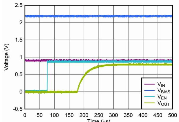
Figure 6-16. Start-Up With  $V_{IN}$  and  $V_{BIAS}$  Before  $V_{EN}$
