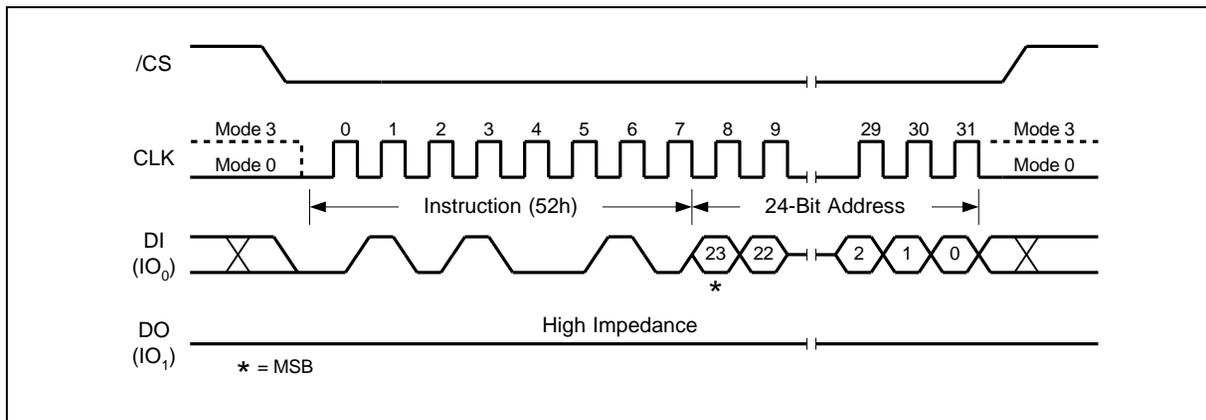
Figure 20. 32KB Block Erase Instruction Sequence Diagram
