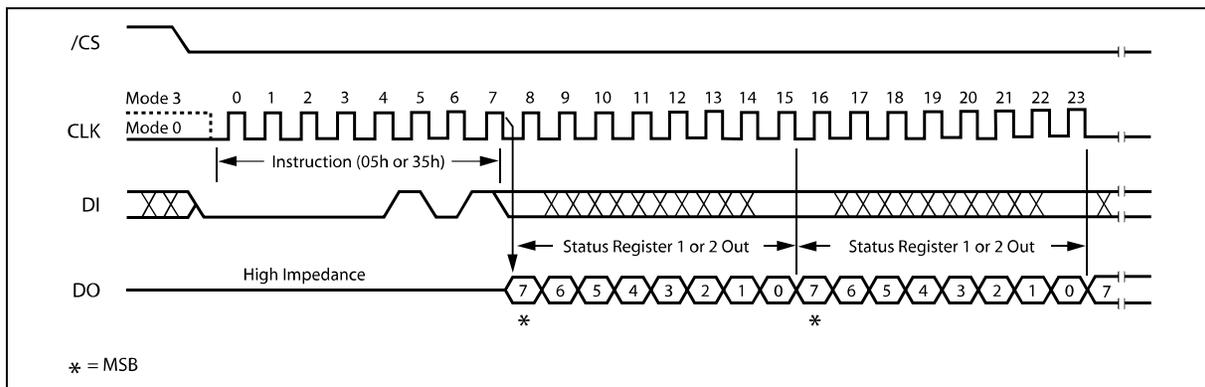
Figure 7. Read Status Register Instruction Sequence Diagram
