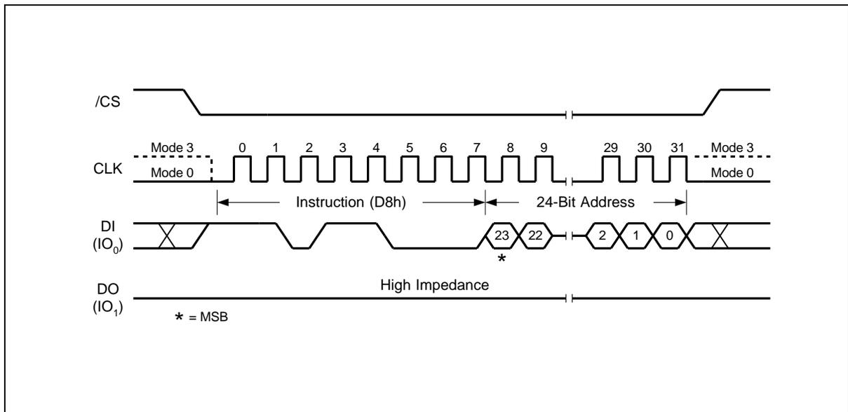
Figure 21. 64KB Block Erase Instruction Sequence Diagram
