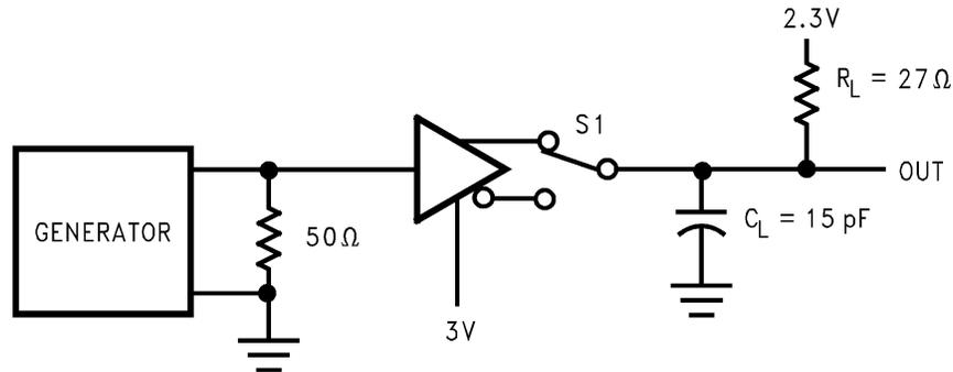
(2) The input pulse is supplied by a generator having the following characteristics: PRR = 1.0 MHz, 50% duty cycle, t<sub>r</sub> ≤ 6.0 ns, t<sub>f</sub> ≤ 6.0 ns, Z<sub>O</sub> = 50Ω.
