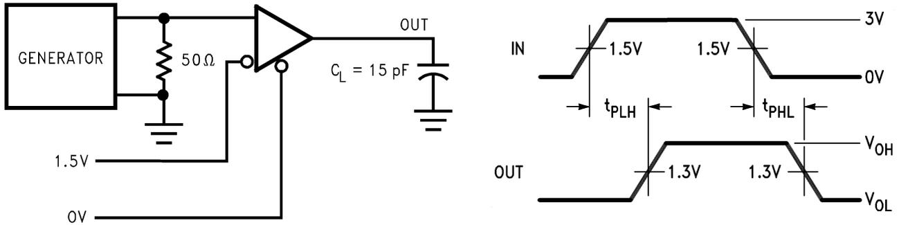
Figure 7. Receiver Propagation Delay Times<sup>(5)(6)</sup>
