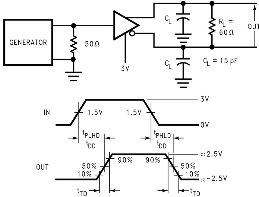
$$t_{\text{SKEW}} = |t_{\text{PLHD}} - t_{\text{PHLD}}|$$
