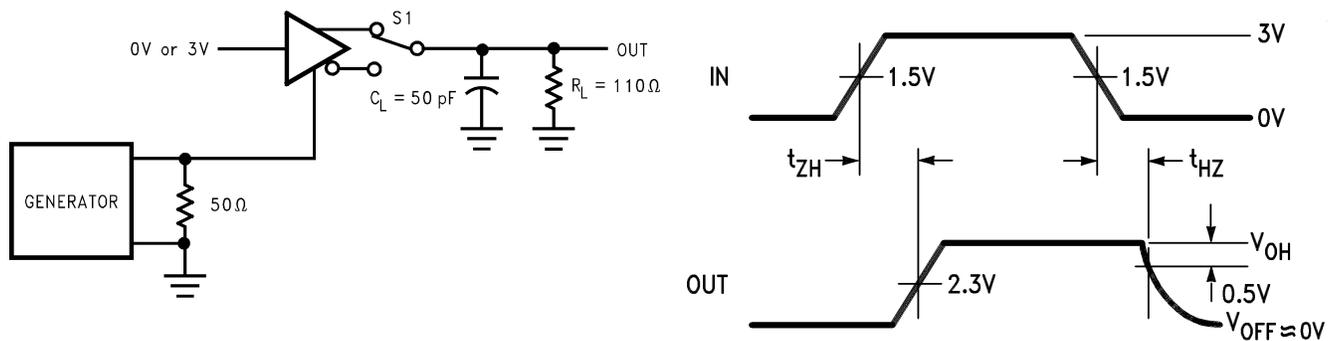
Figure 5. Driver Enable and Disable Times ( $t_{ZH}$ ,  $t_{HZ}$ )<sup>(2)(4)(3)</sup>
