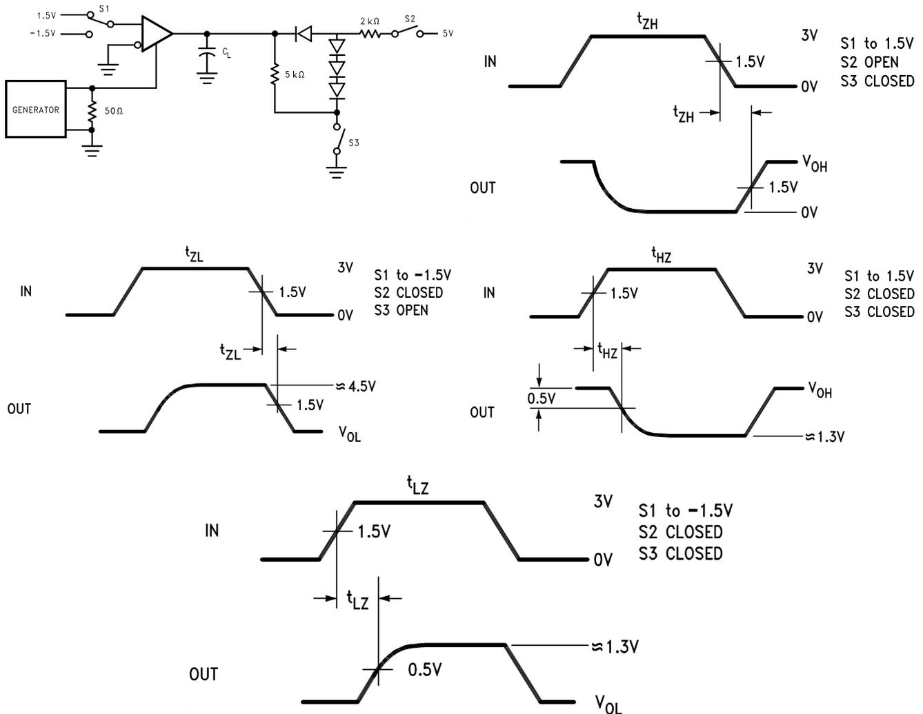
Figure 8. Receiver Enable and Disable Times<sup>(8)(9)(10)</sup>
