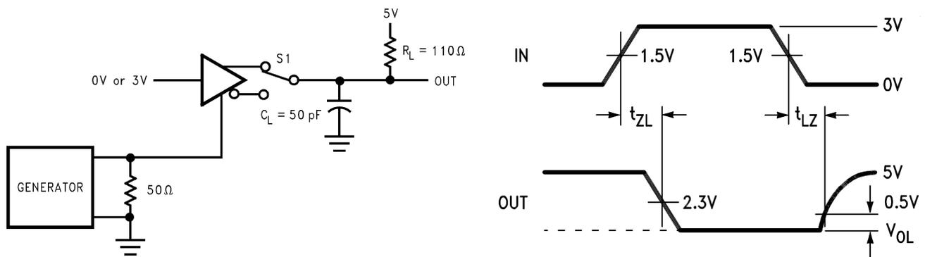
Figure 6. Driver Enable and Disable Times ( $t_{ZL}$ ,  $t_{LZ}$ ,  $t_{LZL}$ )<sup>(5)(6)(7)</sup>
