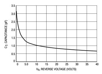
Figure 3. Typical Capacitance
