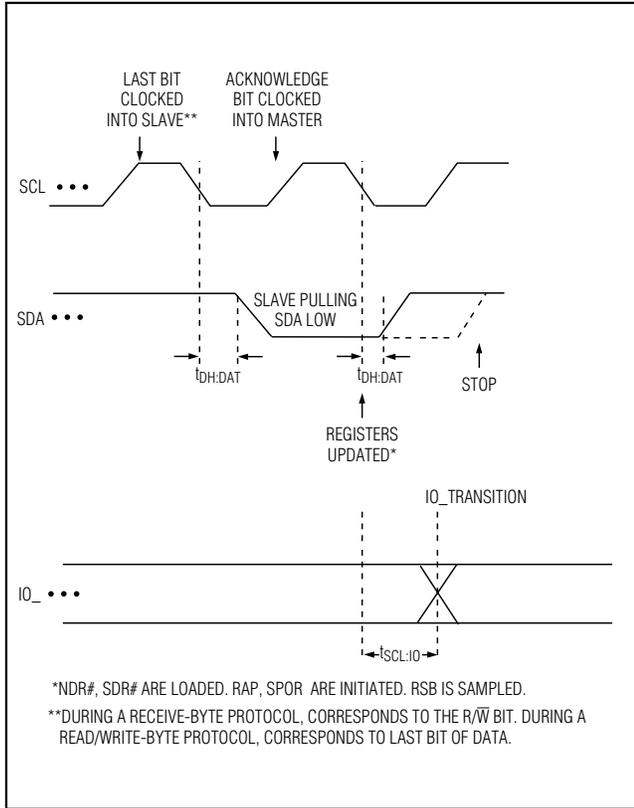
Figure 5. Registers/IO<sub>0</sub> Update Timing Diagram
