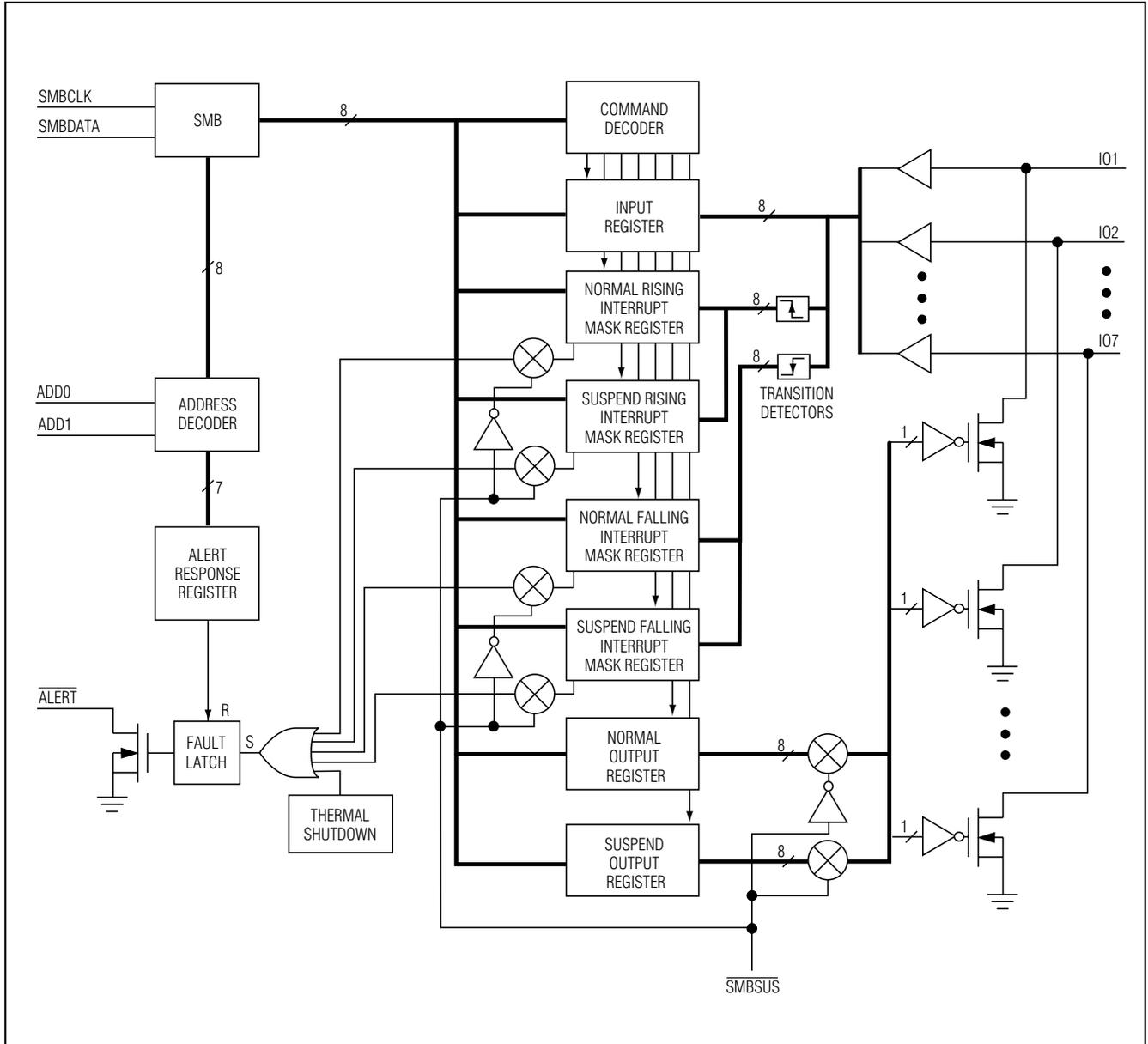
Figure 1. Functional Diagram
