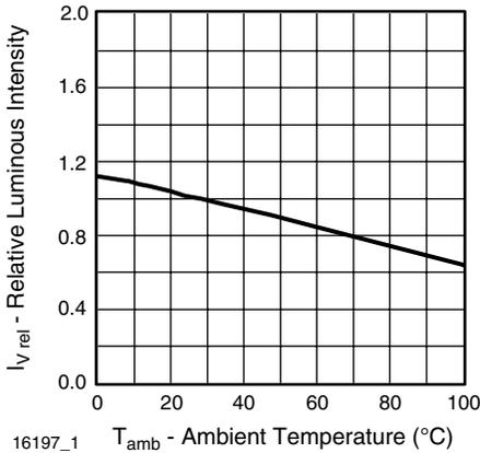
Figure 5. Rel. Luminous Intensity vs. Ambient Temperature
