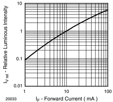
Figure 2. Relative Luminous Intensity vs. Forward Current
