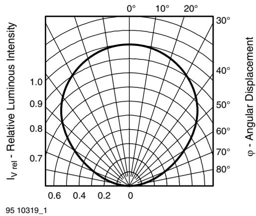
Figure 8. Rel. Luminous Intensity vs. Angular Displacement
