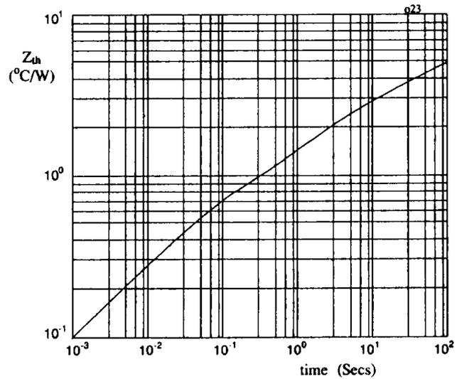
Fig 2. Transient thermal impedance characteristic per leg
