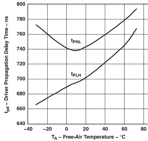
Figure 2. Driver Propagation Delay Time vs Free-Air Temperature
