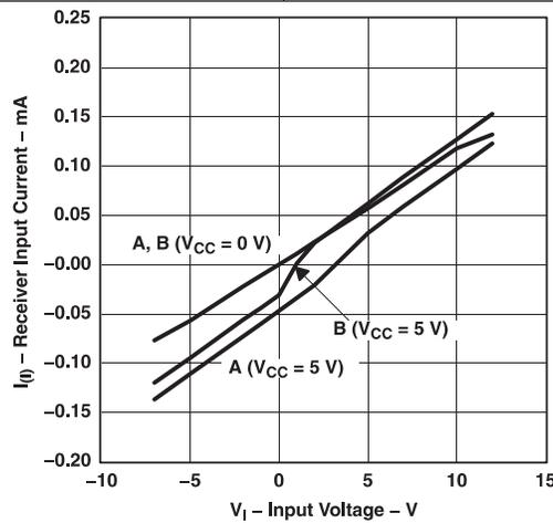
Figure 5. Receiver Input Current vs Input Voltage
