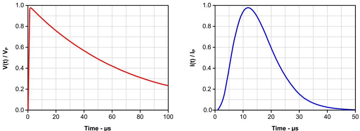
**Figure 18. Open-Circuit Voltage and Short-Circuit Current Waveforms**
