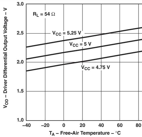
Figure 1. Driver Differential Output Voltage vs Free-Air Temperature
