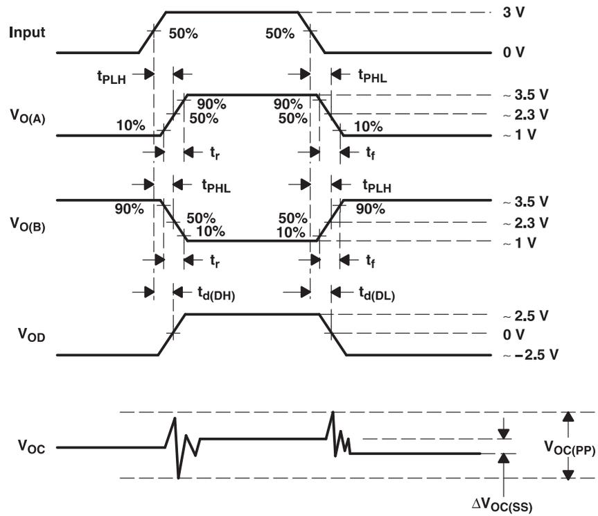
Figure 9. Driver Timing, Voltage, and Current Waveforms
