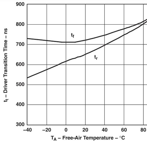
Figure 3. Driver Transition Time vs Free-Air Temperature
