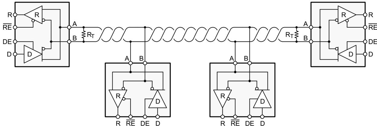
**Figure 16. Typical RS-485 Network With Half-Duplex Transceivers**
