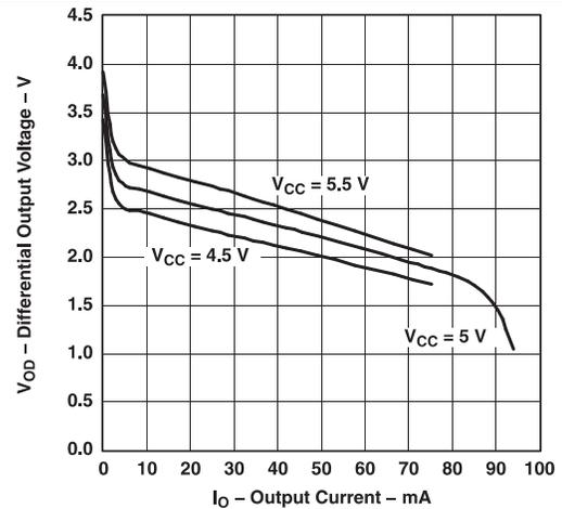
Figure 4. Differential Output Voltage vs Output Current
