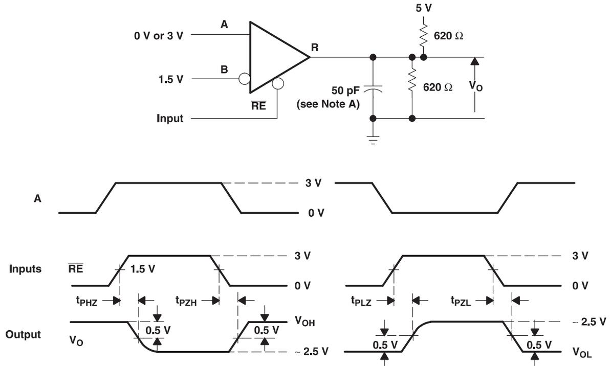
A. This value includes probe and jig capacitance ( $\pm 10\%$ ).
