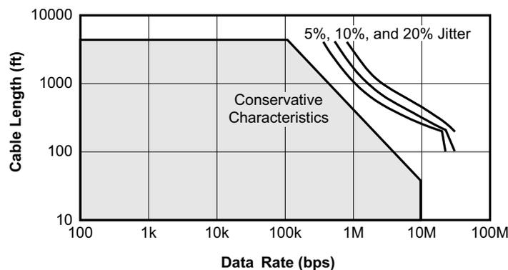
**Figure 17. Cable Length vs Data Rate Characteristic**
