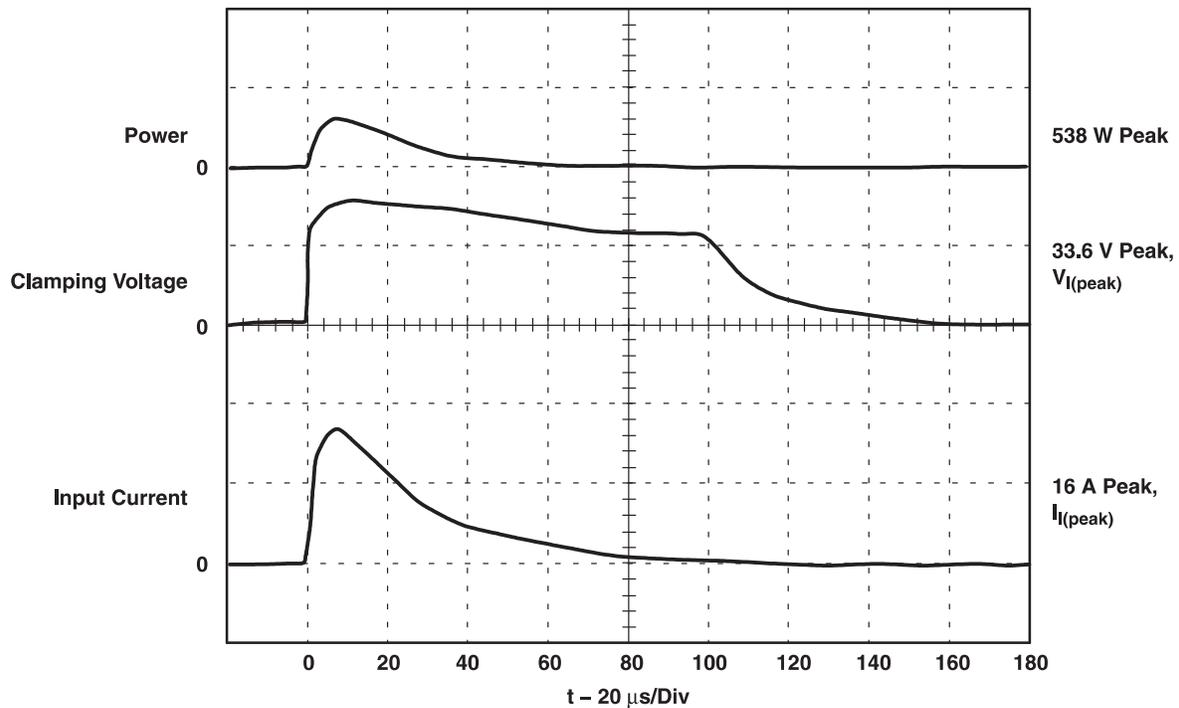
**Figure 20. Typical Surge Waveform Measured at Pins 5 and 7**
