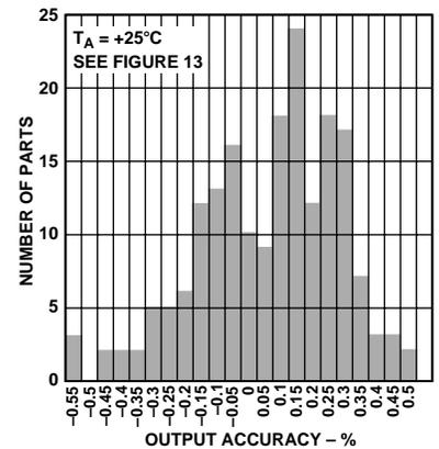
Figure 12. Output Accuracy Distribution,  $V_{OUT} = 2.0\text{ V}$
