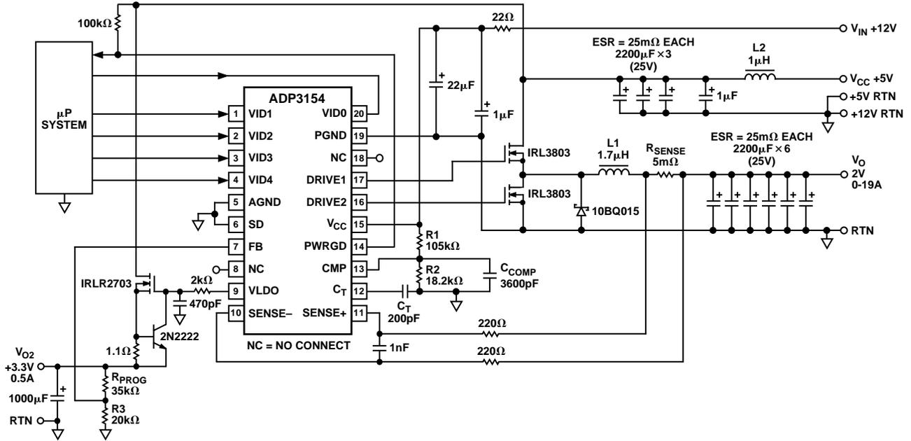
Figure 2. Typical VRM8.2/8.3/8.4 Compliant Core DC/DC Converter Circuit
