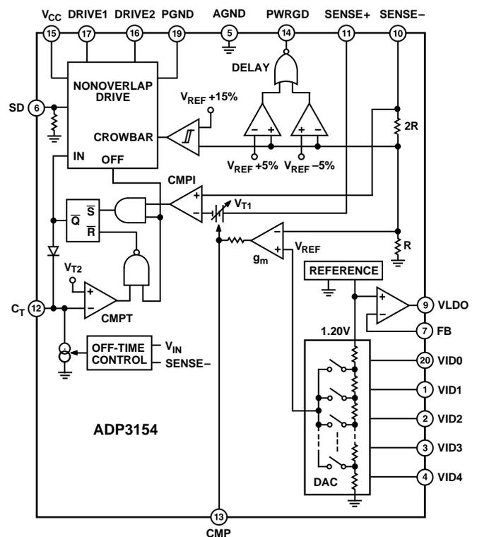
The ADP3154 contains a linear regulator controller that is designed to drive an external N-channel MOSFET. This linear regulator is used to generate the auxiliary voltages (AGP, GTL, etc.) required in most motherboard designs, and has been designed to provide a high bandwidth load-transient response. A pair of external feedback resistors sets the linear regulator output voltage.
