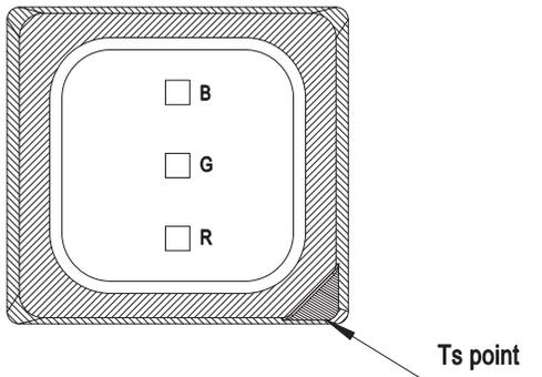
$T_S$  can be easily measured by mounting a thermocouple on the soldering joint as shown in preceding figure, while  $R_{\theta J-S}$  is provided in the data sheet. Verify the  $T_S$  of the LED in the final product to ensure that the LEDs are operating within all maximum ratings stated in the data sheet.
