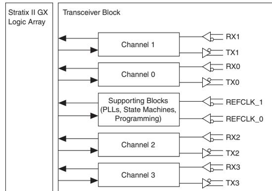
Each Stratix II GX transceiver channel consists of a transmitter and receiver. The transceivers are grouped in four and share PLL resources. Each transmitter has access to one of two PLLs. The transmitter contains the following:
