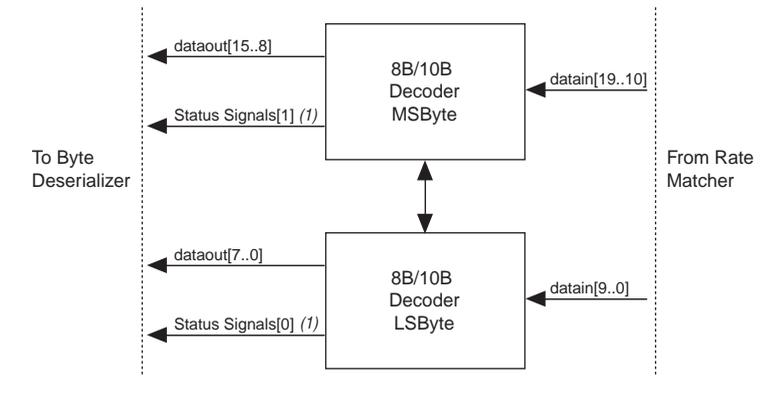
The 8B/10B decoder in single-width mode translates the 10-bit encoded data into the 8-bit equivalent data or control code. The 10-bit code received must be from the supported Dx.y or Kx.y list with the proper disparity or error flags asserted. All 8B/10B control signals, such as disparity error or control detect, are pipelined with the data and edge-aligned with the data. Figure 2–22 shows how the 10-bit symbol is decoded in the 8-bit data + 1-bit control indicator.
