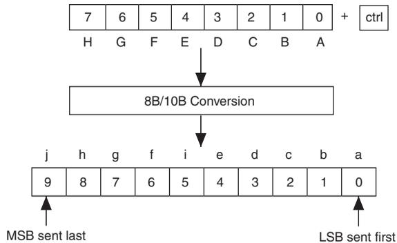
In single-width mode, the 8B/10B encoder generates a 10-bit code group from the 8-bit data and 1-bit control identifier. In double-width mode, there are two 8B/10B encoders that are cascaded together and generate a 20-bit ( $2 \times 10$ -bit) code group from the 16-bit ( $2 \times 8$ -bit) data + 2-bit ( $2 \times 1$ -bit) control identifier. [Figure 2-6](#) shows the 20-bit encoding process. The 8B/10B encoder conforms to the IEEE 802.3 1998 edition standards.
