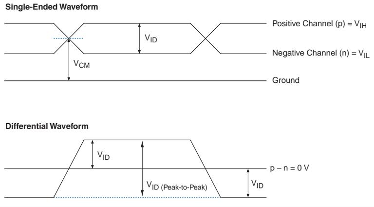
**Figure 4-7. Transmitter Output Waveforms for Differential I/O Standards**
