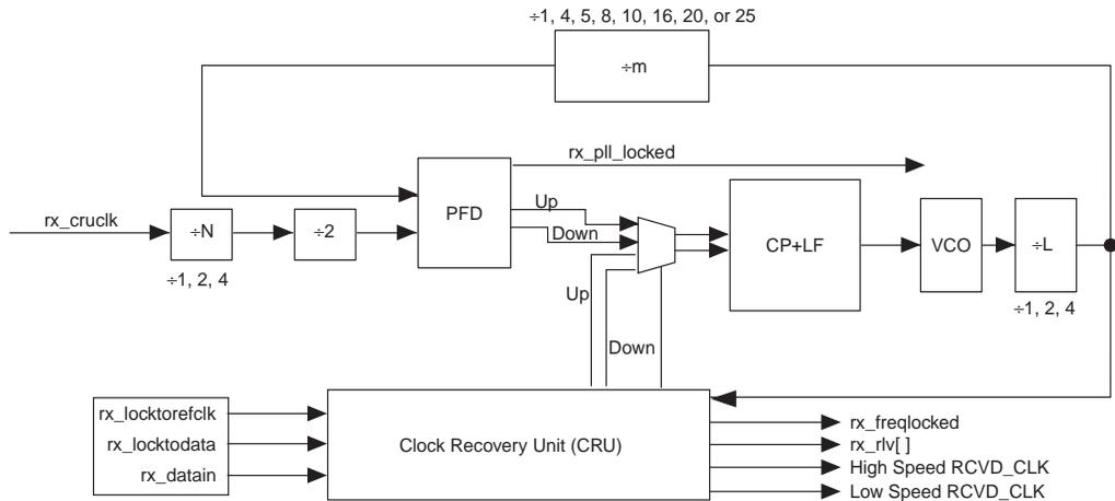
The receiver PLLs and CRUs can support frequencies up to 6.375 Gbps. The input clock frequency is limited to the full clock range of 50 to 622 MHz but only when using REFCLK0 or REFCLK1. An optional RX\_PLL\_LOCKED port is available to indicate whether the PLL is locked to the reference clock. The receiver PLL has a programmable loop bandwidth which can be set to low, medium, or high. The Quartus II software can statically set the loop bandwidth parameter.
