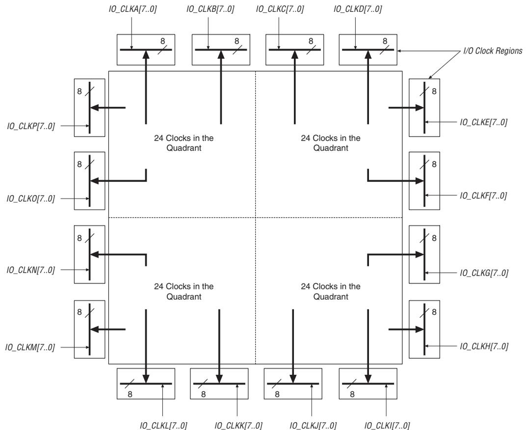
You can use the Quartus II software to control whether a clock input pin drives either a global, regional, or dual-regional clock network. The Quartus II software automatically selects the clocking resources if not specified.
