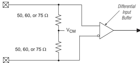
If a design uses external termination, the receiver must be externally terminated and biased to 0.85 V or 1.2 V. [Figure 2–14](#) shows an example of an external termination and biasing circuit.
