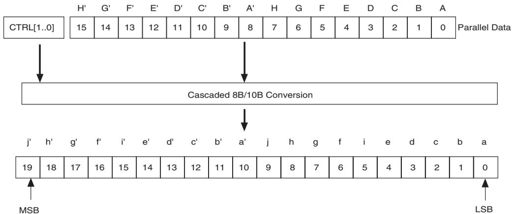
Upon power on or reset, the 8B/10B encoder has a negative disparity which chooses the 10-bit code from the RD-column. However, the running disparity can be changed via the `tx_forcedisp` and `tx_dispsval` ports.
