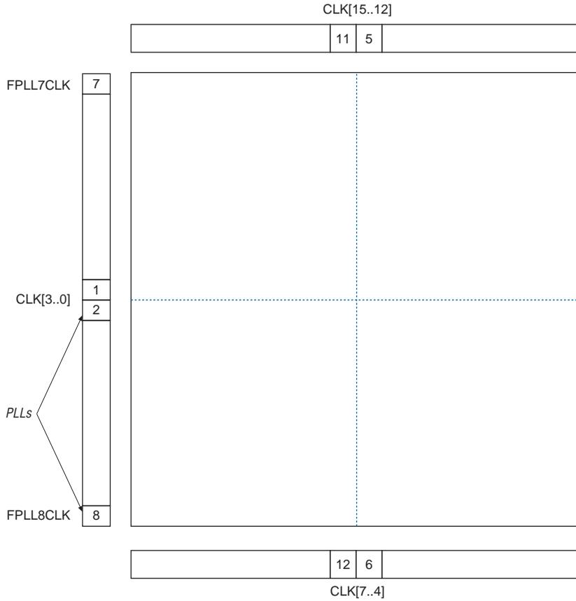
Figures 2–71 and 2–72 shows global and regional clocking from the fast PLL outputs and the side clock pins. The connections to the global and regional clocks from the fast PLL outputs, internal drivers, and the CLK pins on the left side of the device are shown in Table 2–27.
