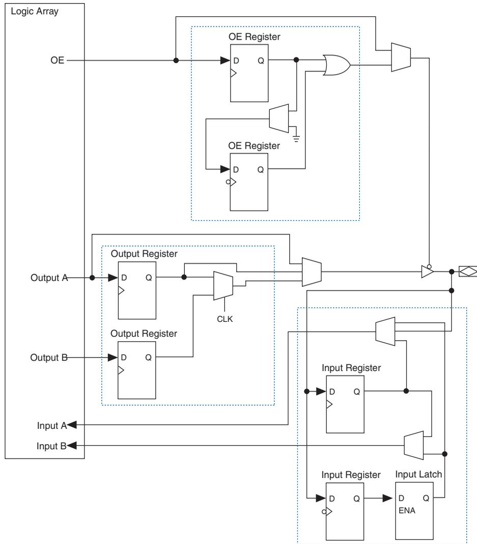
The IOEs are located in I/O blocks around the periphery of the Stratix II GX device. There are up to four IOEs per I/O block and four IOEs per column I/O block. The row I/O blocks drive row, column, or direct link interconnects. The column I/O blocks drive column interconnects.
