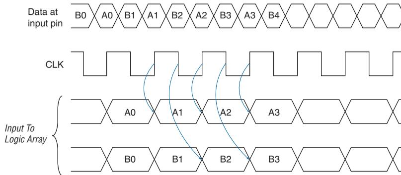
When using the IOE for DDR outputs, the two output registers are configured to clock two data paths from ALMs on rising clock edges. These output registers are multiplexed by the clock to drive the output pin at a  $\times 2$  rate. One output register clocks the first bit out on the clock high time, while the other output register clocks the second bit out on the clock low time. [Figure 2–84](#) shows the IOE configured for DDR output. [Figure 2–85](#) shows the DDR output timing diagram.
