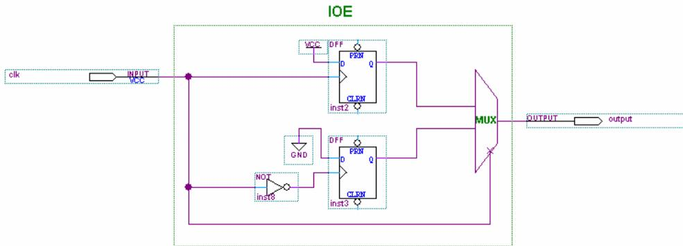
When an FPGA PLL generates the internal clock, the PLL output clocks the IOE block. As the PLL only monitors the positive edge of the reference clock input and internally re-creates the output clock signal, any DCD present on the reference clock is filtered out. Therefore, the DCD for a DDIO output with PLL in the clock path is better than the DCD for a DDIO output without PLL in the clock path.
