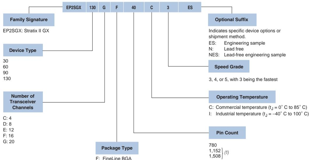
(1) Product code notations for ES silicon for all EP2SGX130 family members (standard and lead free) and EP2SGX90 (lead free) use the following codings to denote pin count: 35 for 1152-pin devices and 40 for 1508-pin devices
