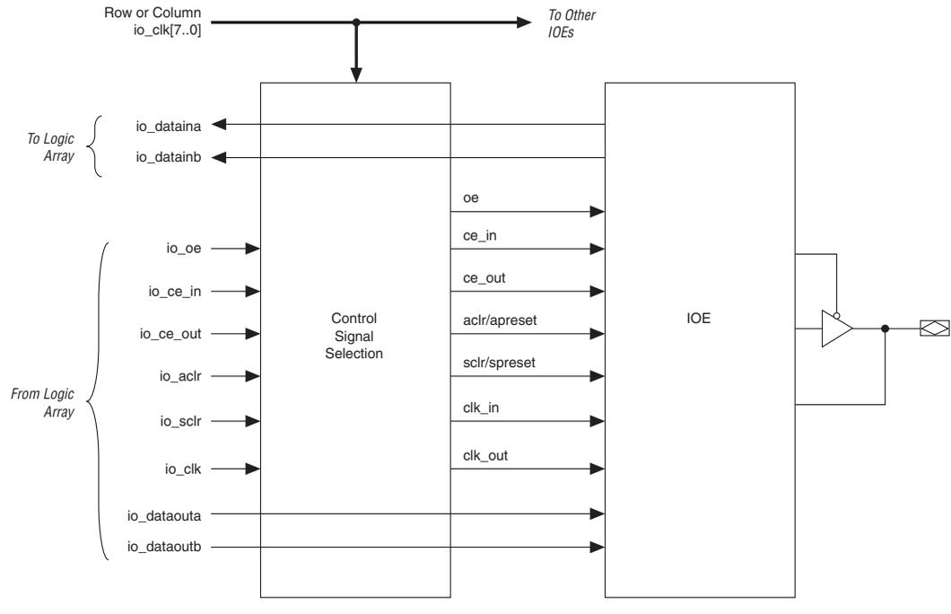
Each IOE contains its own control signal selection for the following control signals:  $oe$ ,  $ce\_in$ ,  $ce\_out$ ,  $aclr/apreset$ ,  $sclr/spreset$ ,  $clk\_in$ , and  $clk\_out$ . Figure 2–80 illustrates the control signal selection.
