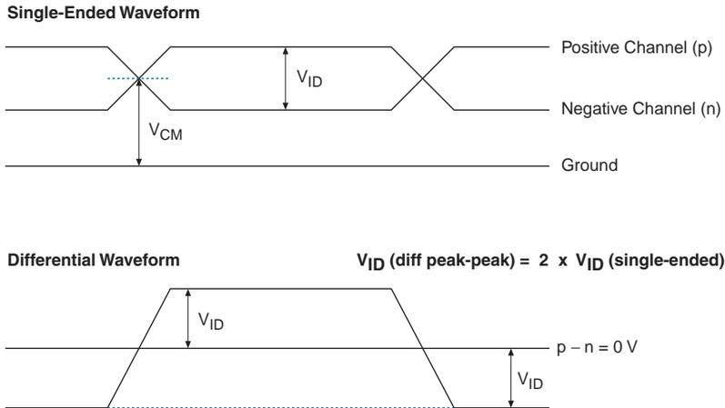
**Figure 4–4. Transmitter Output Waveform**
