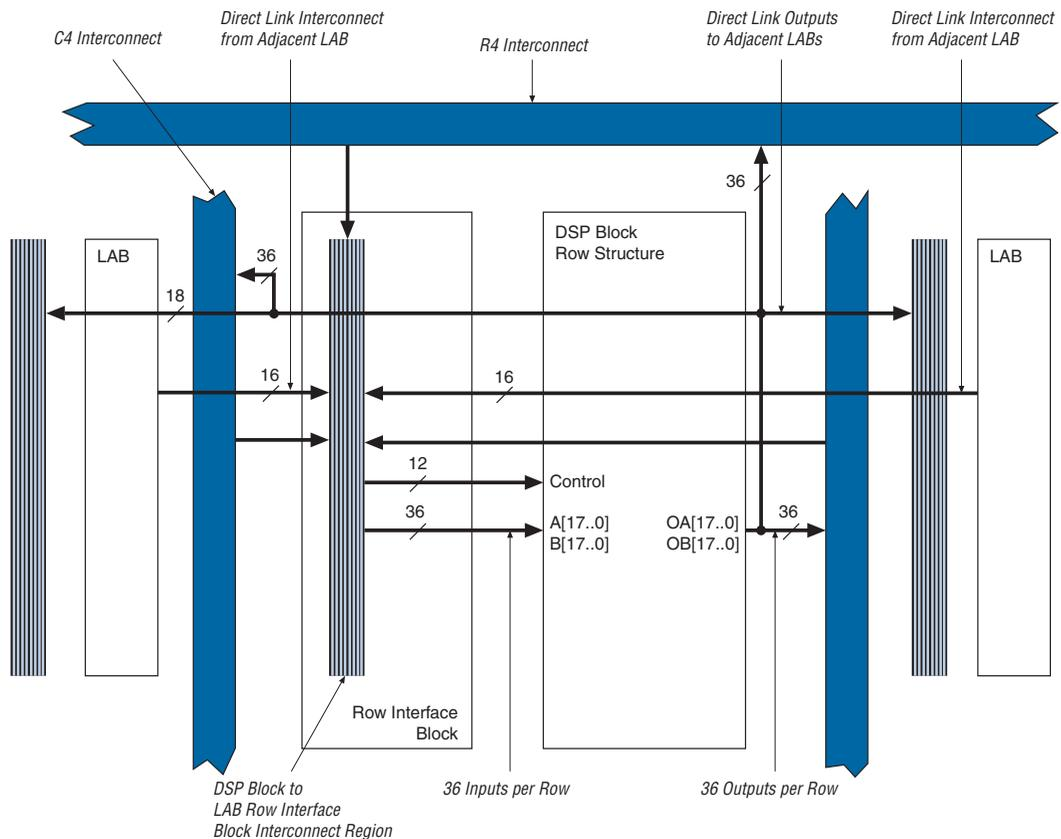
A bus of 44 control signals feeds the entire DSP block. These signals include clocks, asynchronous clears, clock enables, signed and unsigned control signals, addition and subtraction control signals, rounding and saturation control signals, and accumulator synchronous loads. The clock signals are routed from LAB row clocks and are generated from specific LAB rows at the DSP block interface. The LAB row source for control signals, data inputs, and outputs is shown in [Table 2–23](#).
