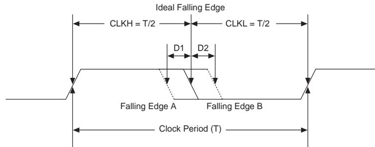
DCD expressed in absolute derivation, for example, D1 or D2 in [Figure 4–11](#), is clock-period independent. DCD can also be expressed as a percentage, and the percentage number is clock-period dependent. DCD as a percentage is defined as:
