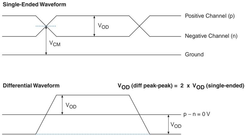
**Figure 4–5. Maximum Receiver Input Pin Voltage**
