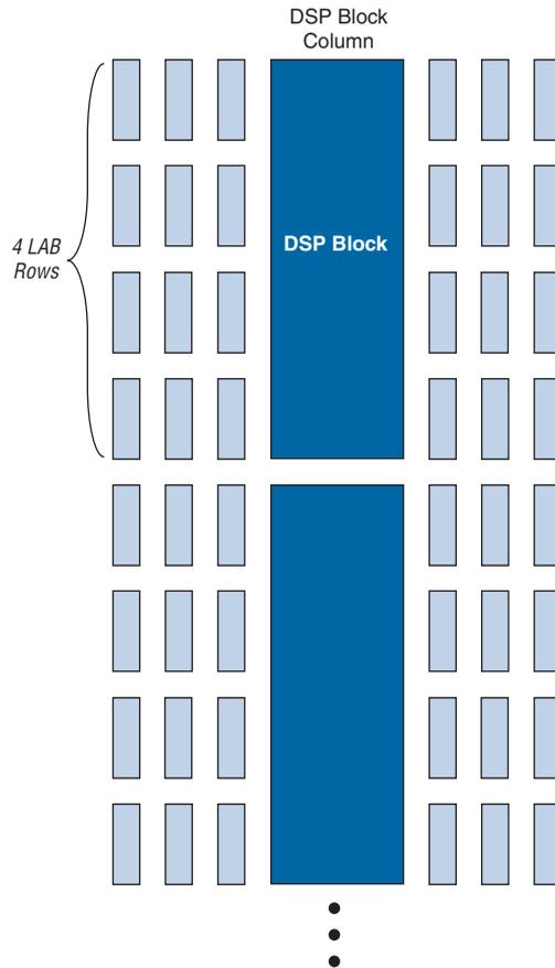
Table 2–21 shows the number of DSP blocks in each Stratix II GX device. DSP block multipliers can optionally feed an adder/subtractor or accumulator in the block, depending on the configuration, which makes routing to ALMs easier, saves ALM routing resources, and increases performance because all connections and blocks are in the DSP block.
