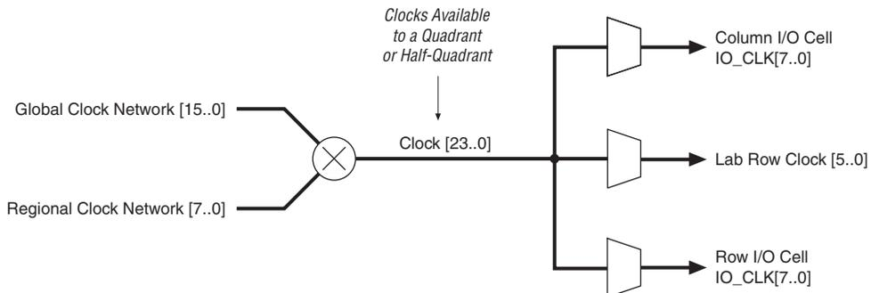
IOE clocks have row and column block regions that are clocked by 8 I/O clock signals chosen from the 24 quadrant clock resources. Figures 2-65 and 2-66 show the quadrant relationship to the I/O clock regions.
