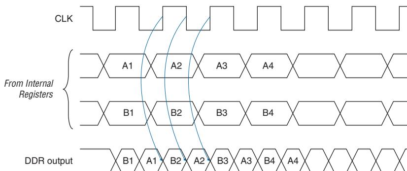
The Stratix II GX IOE operates in bidirectional DDR mode by combining the DDR input and DDR output configurations. The negative-edge-clocked OE register holds the  $\text{OE}$  signal inactive until the falling edge of the clock to meet DDR SDRAM timing requirements.
