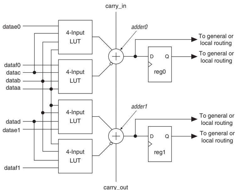
While operating in arithmetic mode, the ALM can support simultaneous use of the adder's carry output along with combinational logic outputs. In this operation, the adder output is ignored. This usage of the adder with the combinational logic output provides resource savings of up to 50% for functions that can use this ability. An example of such functionality is a conditional operation, such as the one shown in [Figure 2–42](#). The equation for this example is:
