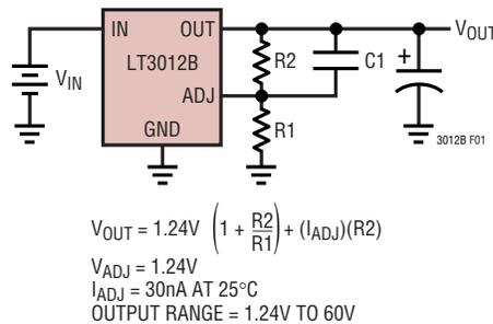
Figure 1. Adjustable Operation
