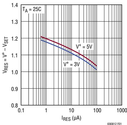
Figure 1.  $V^+ - V_{SET}$  Variation with  $I_{RES}$
