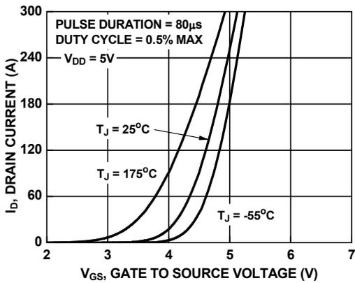
Figure 7. Transfer Characteristics
