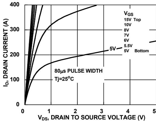
Figure 9. Saturation Characteristics
