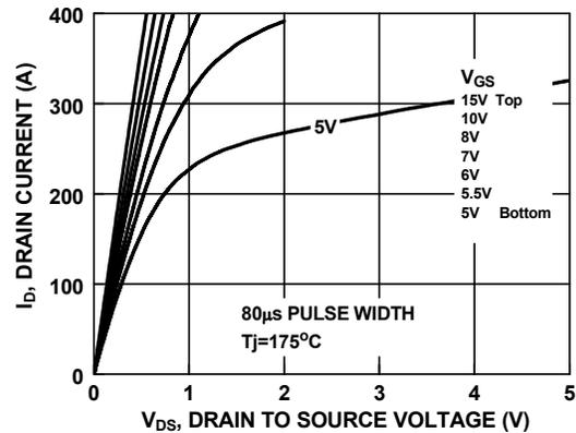
Figure 10. Saturation Characteristics
