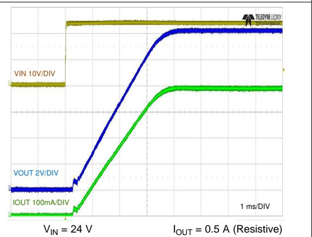
Figure 18. Full-Load Start-up with VIN
