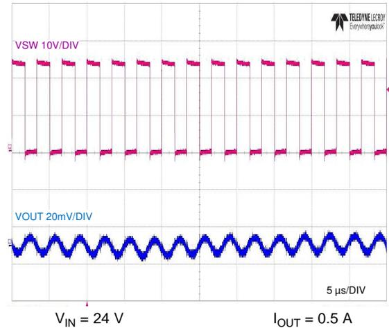
Figure 26. Full-Load Switching
