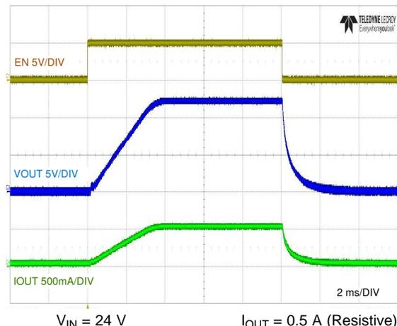
Figure 20. Full-Load Start-up and Shutdown with EN/UVLO
