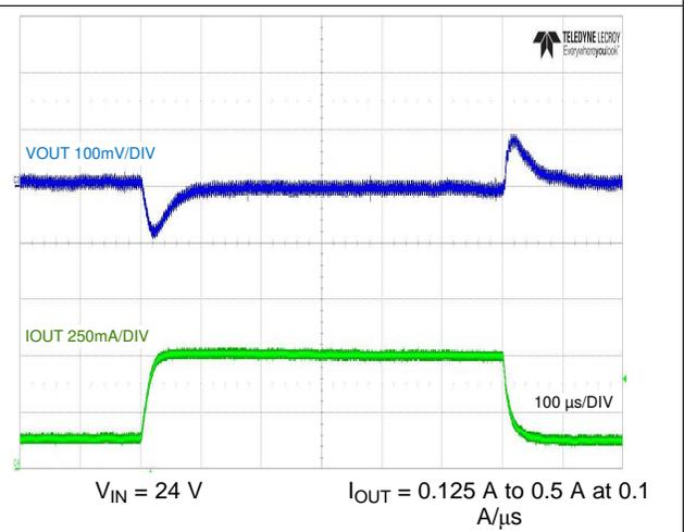
Figure 16. Load Step Response
