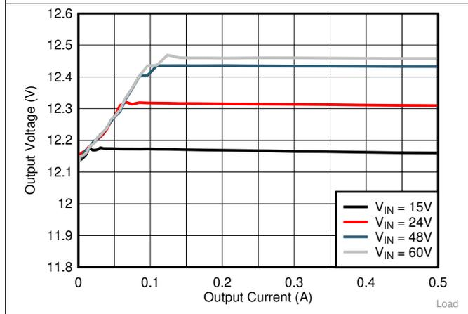
Figure 15. Load and Line Regulation Performance
