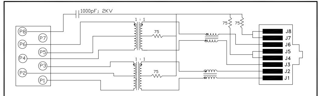
: 350uH MIN. @ 0.1V, 100KHz, 8mA DC Bias : 350uH MIN. @ 0.1V, 100KHz, 8mA DC Bigs
