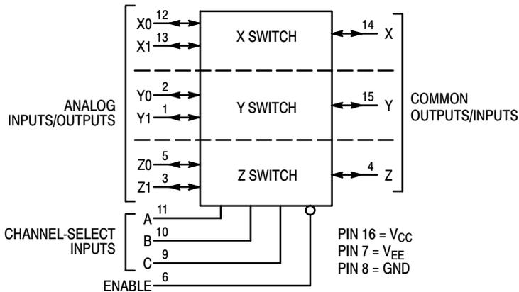
NOTE: This device allows independent control of each switch. Channel-Select Input A controls the X-Switch, Input B controls the Y-Switch and Input C controls the Z-Switch
