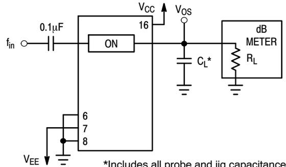
**Figure 6. Maximum On Channel Bandwidth, Test Set-Up**
