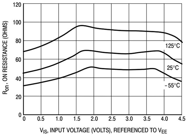
Figure 1c. Typical On Resistance,  $V_{CC} - V_{EE} = 4.5 \text{ V}$
