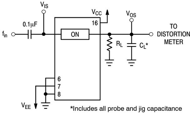
Figure 14a. Total Harmonic Distortion, Test Set-Up
