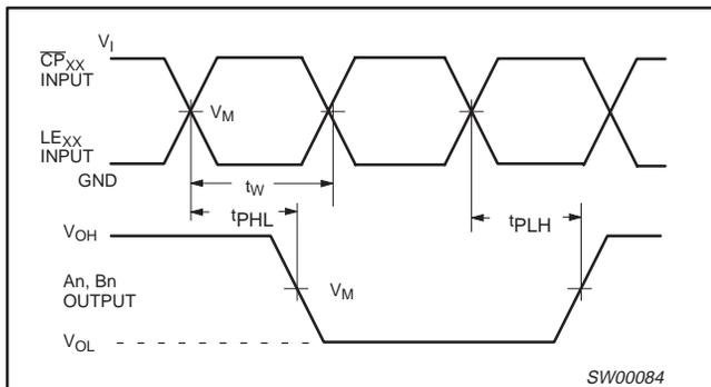
**Waveform 2. Latch enable input (LE<sub>AB</sub>, LE<sub>BA</sub>) and clock pulse input (CP<sub>AB</sub>, CP<sub>BA</sub>) to output (An, Bn) propagation delays and latch enable pulse width**
