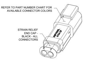
RECEPTACLE, 2 PIN, AT SERIES, STRAIN RELIEF END CAP
