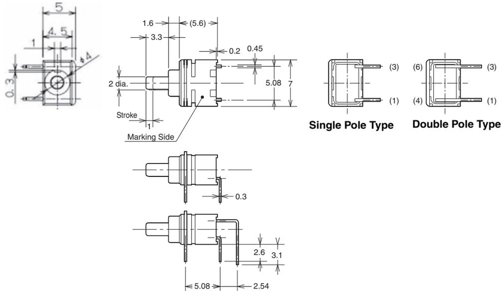
Note: Unless otherwise specified, a tolerance of ±0.4 mm applies to all dimensions.
