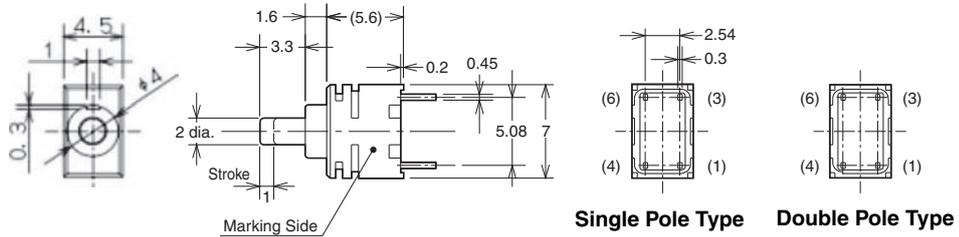
Note: NO.(4) and (6) terminals in the SPDT models are dummies to support the Switch case.
