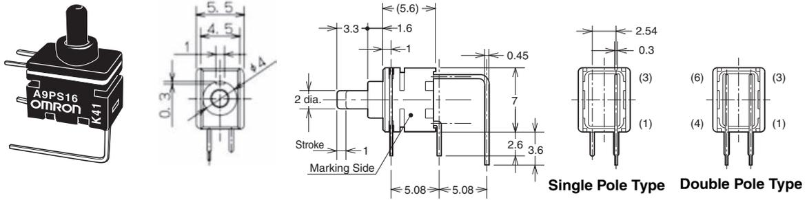
Note: Unless otherwise specified, a tolerance of ±0.4 mm applies to all dimensions.
