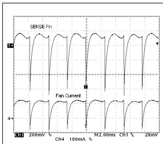
**FIGURE 7-6:** Typical Fan Current and Sense Pin Waveforms.
