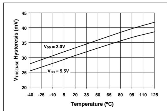
**FIGURE 2-11:** Sense Threshold ( $V_{THSENSE}$ ) Hysteresis vs. Temperature.
