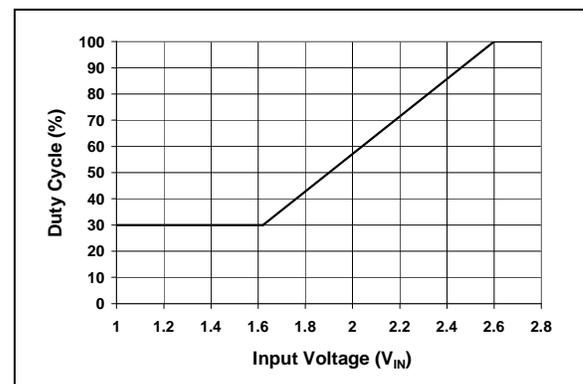
**FIGURE 4-5:** PWM Duty Cycle vs.  $V_{IN}$  Voltage (Typical).
