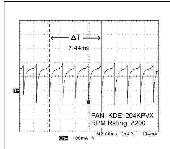
**FIGURE 7-9:** Four Current Pulses Per Revolution Fan.
