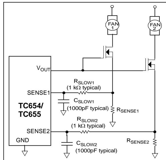
**FIGURE 7-12:** FET Drive with  $R_{SLOW}/C_{SLOW}$  Sense Scheme.
