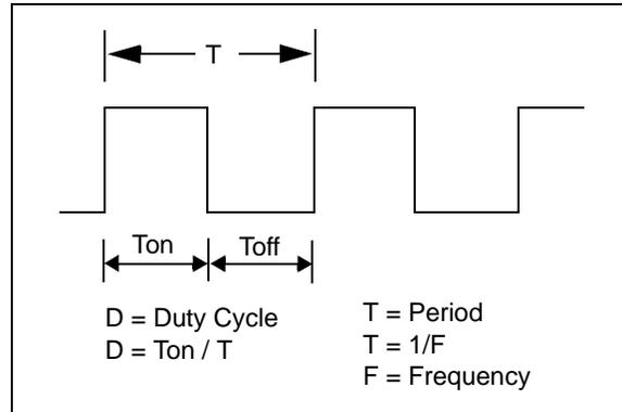
**FIGURE 4-2:** Duty Cycle Of A PWM Waveform.
