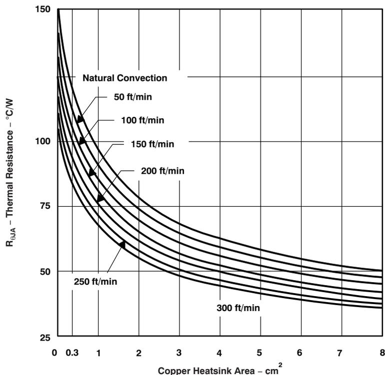
Figure 27. Thermal Resistance vs Copper Heatsink Area
