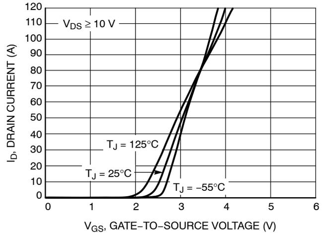
Figure 2. Transfer Characteristics
