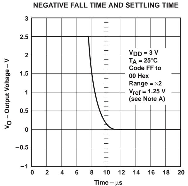
NOTE A: Fall time = 4.25  $\mu$ s, negative slew rate = 0.46 V/ $\mu$ s, settling time = 8.5  $\mu$ s.
