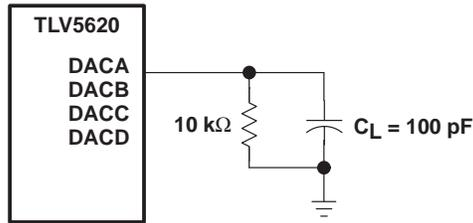
Figure 6. Slew, Settling Time, and Linearity Measurements
