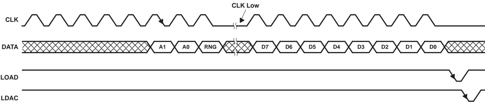
Figure 4. LDAC Controlled Update Using 8-Bit Serial Word
