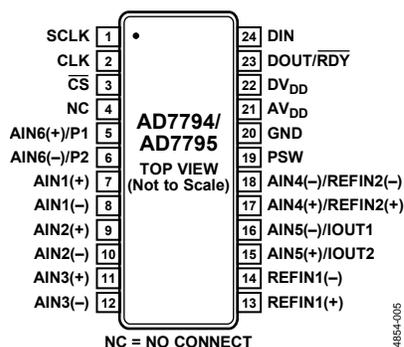
Figure 5. Pin Configuration
