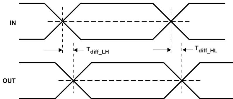
Figure 3. Propagation Delay
