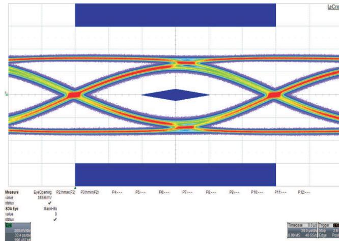
DE= 0dB, EQ = 7dB, Input = 12", Output = 8" + 3m Cable
