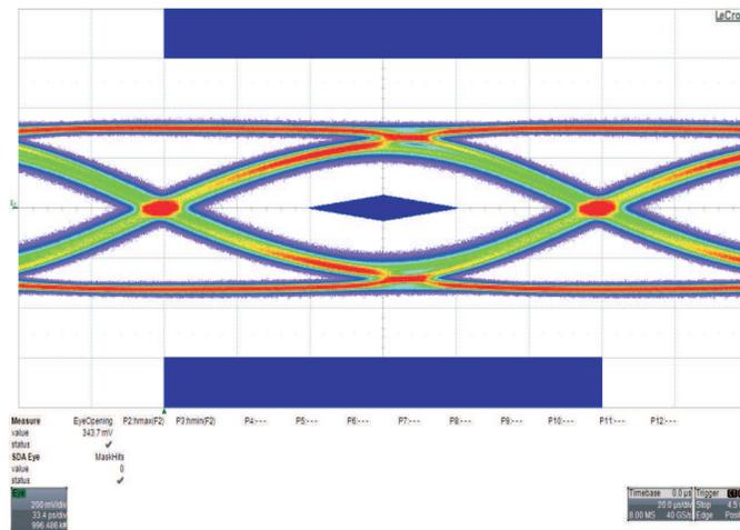
**DE= 0dB, EQ = 0dB, Input = 12", Output = 4" + 3m Cable**
