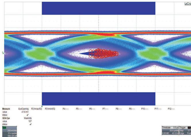
DE= 0dB, EQ = 7dB, Input = 24", Output = 4" + 3m Cable
