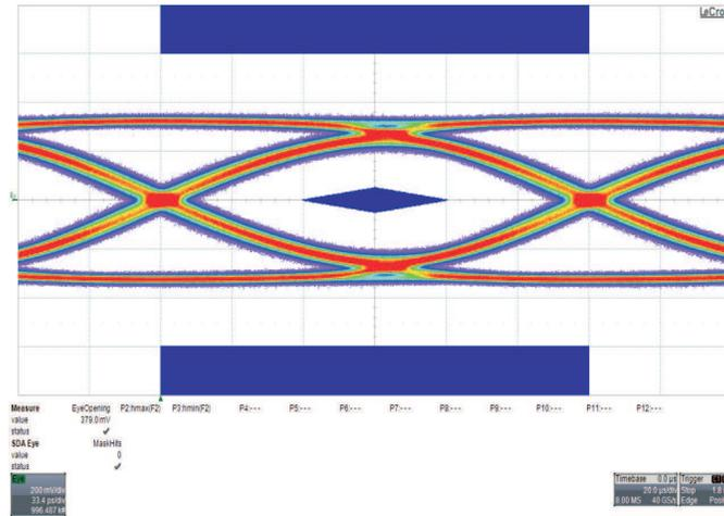
DE= 0dB, EQ = 15dB, Input = 48", Output = 4" + 3m Cable
