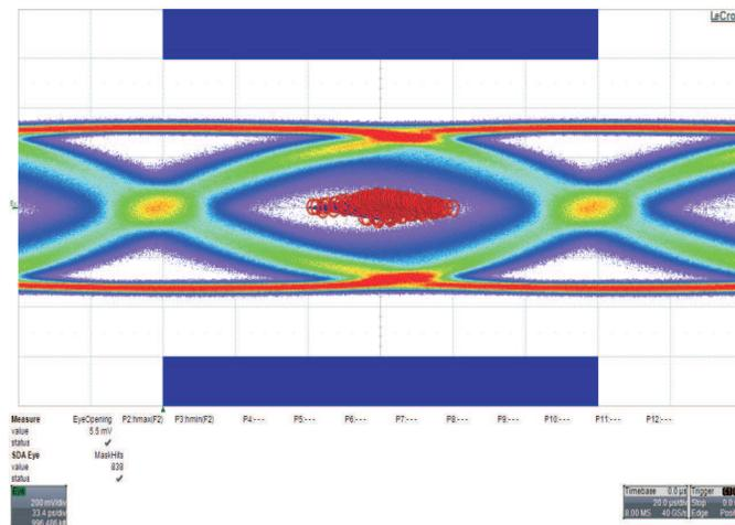
DE= 0dB, EQ = 15dB, Input = 36", Output = 4" + 3m Cable
