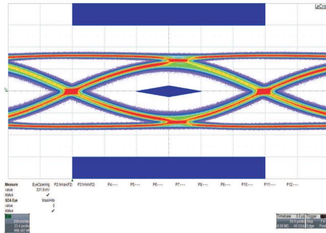
DE= 0dB, EQ = 7dB, Input = 32", Output = 4" + 3m Cable
