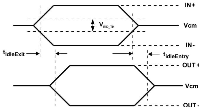
Figure 4. Electrical Idle Mode Exit and Entry Delay
