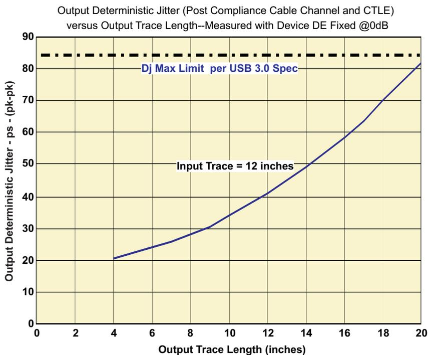
**PLOT #3 FIXED INPUT TRACE WITH VARIABLE OUTPUT TRACE and (No Cable)**
