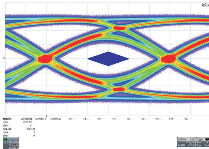
DE= 0dB, EQ = 7dB, Input = 12", Output = 16" + 3m Cable
