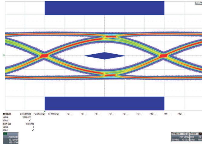
DE= 0dB, EQ = 0dB, Input = 8", Output = 4" + 3m Cable
