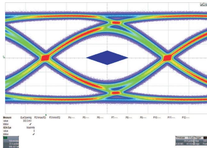
DE= 0dB, EQ = 7dB, Input = 12", Output = 12" + 3m Cable
