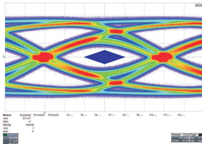
DE= 0dB, EQ = 7dB, Input = 12", Output = 20" + 3m Cable
