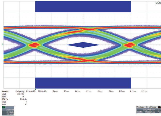
**DE= 0dB, EQ = 0dB, Input = 16", Output = 4" + 3m Cable**
