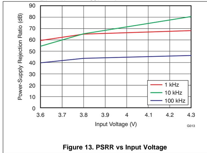
Figure 13. PSRR vs Input Voltage
