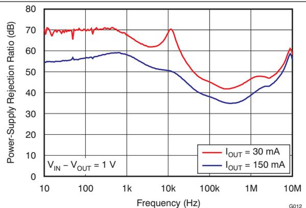
Figure 12. TLV71728PSRR vs Frequency
