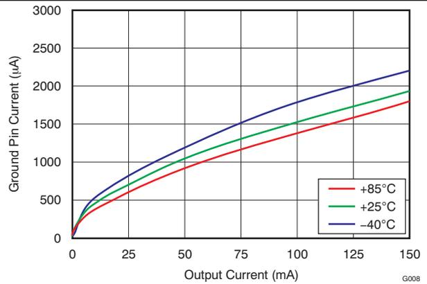
Figure 8. Ground Pin Current vs Output Current
