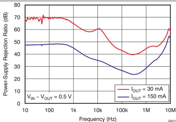
Figure 11. TLV71728PSRR vs Frequency
