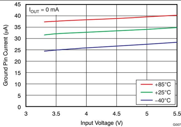
Figure 7. Ground Pin Current vs Input Voltage
