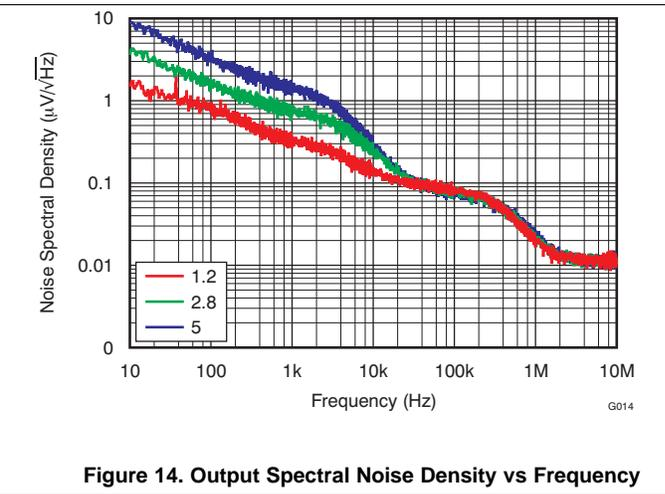
Figure 14. Output Spectral Noise Density vs Frequency
