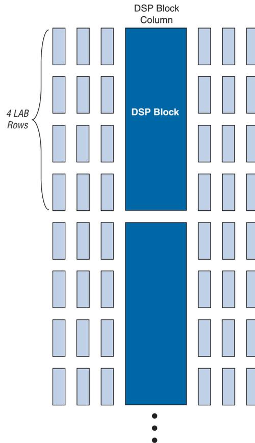
Table 2-13 lists the number of DSP blocks in each Arria GX device. DSP block multipliers can optionally feed an adder/subtractor or accumulator in the block depending on the configuration, which makes routing to ALMs easier, saves ALM routing resources, and increases performance because all connections and blocks are in the DSP block.
