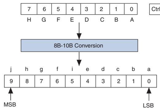
During reset (`tx_digitalreset`), the running disparity and data registers are cleared and the 8B/10B encoder continuously outputs a K28.5 pattern from the RD-column. After out of reset, the 8B/10B encoder starts with a negative disparity (RD-) and transmits three K28.5 code groups for synchronizing before it starts encoding the input data or control character.
