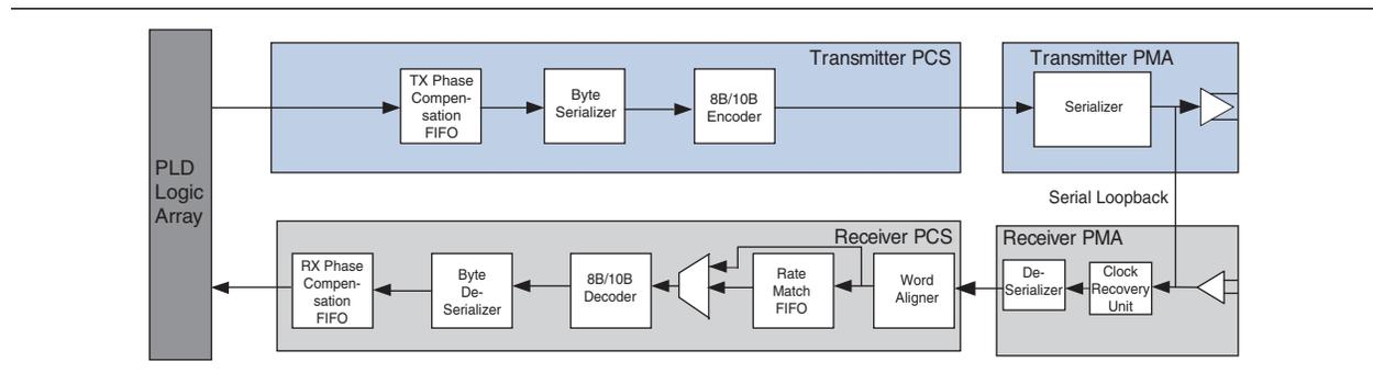
In GIGE and Serial RapidIO modes, you can dynamically put each transceiver channel individually in serial loopback by controlling the `rx_serialloopback` port. A high on the `rx_serialloopback` port puts the transceiver into serial loopback and a low takes the transceiver out of serial loopback.
