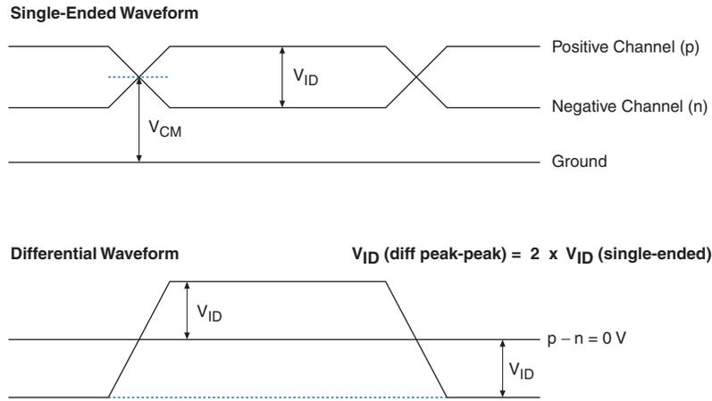
**Figure 4-4.** Transmitter Output Waveform
