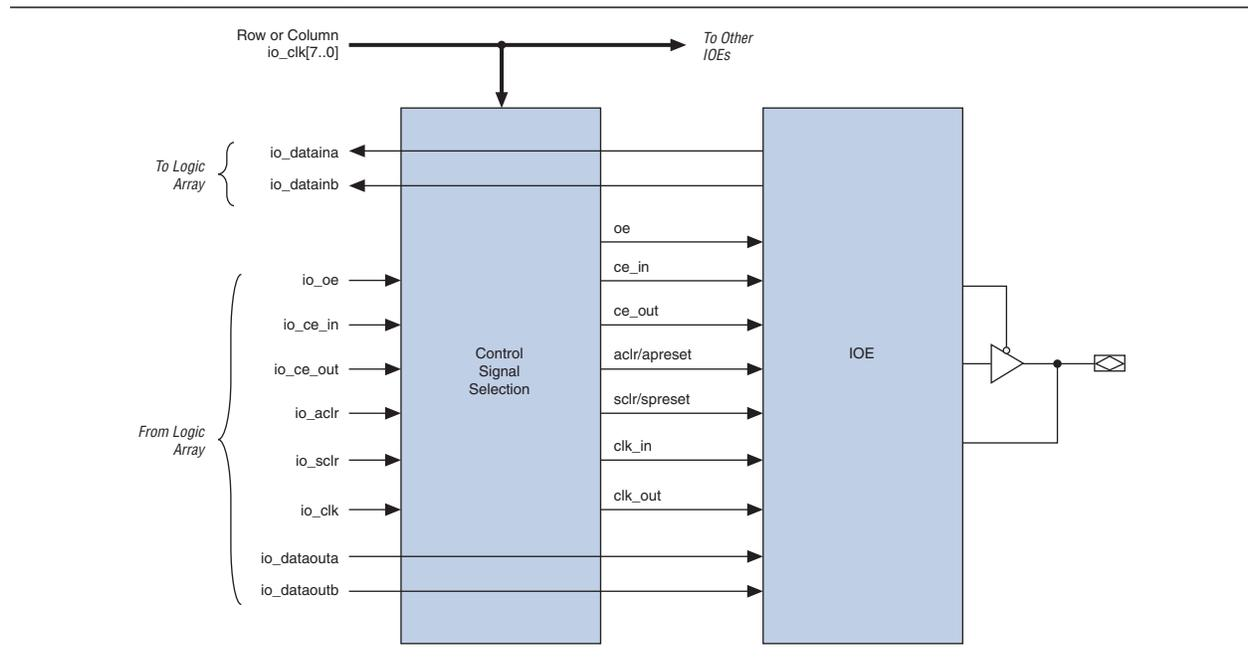
Each IOE contains its own control signal selection for the following control signals: oe, ce\_in, ce\_out, aclr/apreset, sclr/spreset, clk\_in, and clk\_out.
