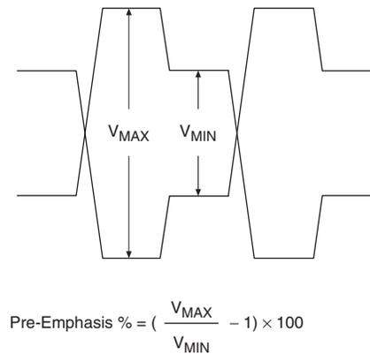
Pre-emphasis percentage is defined as  $(V_{\text{MAX}}/V_{\text{MIN}} - 1) \times 100$ , where  $V_{\text{MAX}}$  is the differential emphasized voltage (peak-to-peak) and  $V_{\text{MIN}}$  is the differential steady-state voltage (peak-to-peak).
