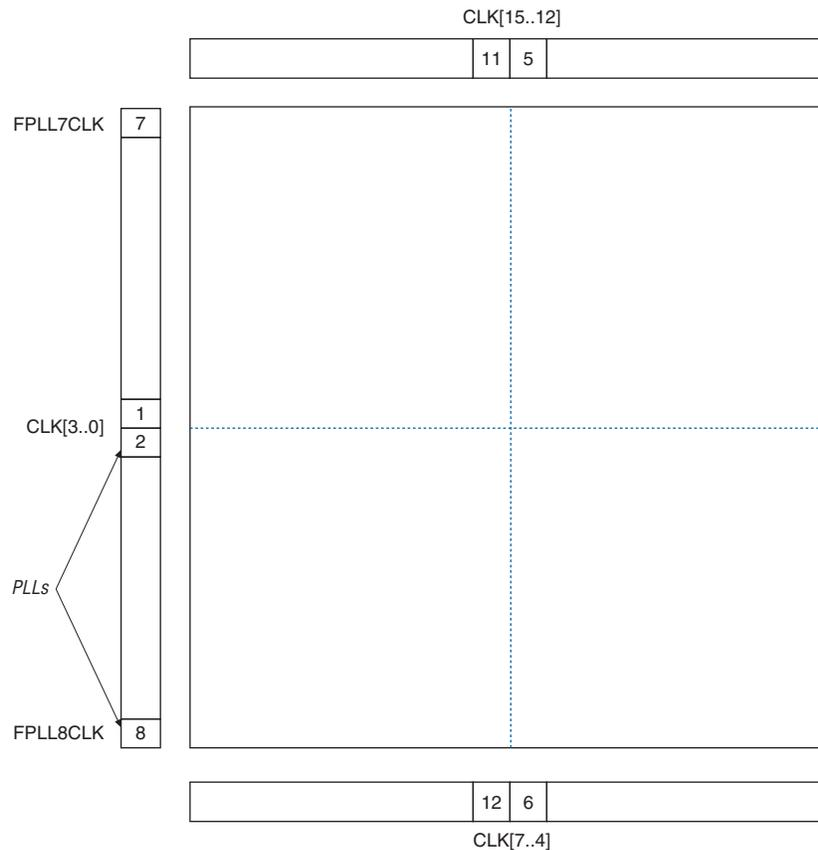
Figure 2-62 and Figure 2-63 shows global and regional clocking from the fast PLL outputs and side clock pins. The connections to the global and regional clocks from the fast PLL outputs, internal drivers, and CLK pins on the left side of the device are shown in Table 2-19.
