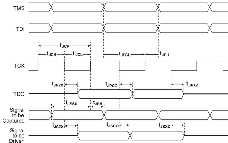
Table 4-123 lists the JTAG timing parameters and values for Arria GX devices.
