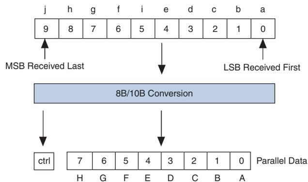
If the received 10-bit code is not a part of valid  $Dx.y$  or  $Kx.y$  code groups, the 8B/10B decoder block asserts an error flag on the `rx_errdetect` port. If the received 10-bit code is detected with incorrect running disparity, the 8B/10B decoder block asserts an error flag on the `rx_disperr` and `rx_errdetect` ports. The error flag signals (`rx_errdetect` and `rx_disperr`) have the same data path delay from the 8B/10B decoder to the PLD-transceiver interface as the bad code group.
