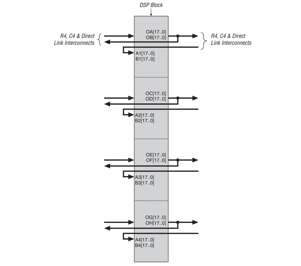
**Figure 2-53.** DSP Block Interface to Interconnect
