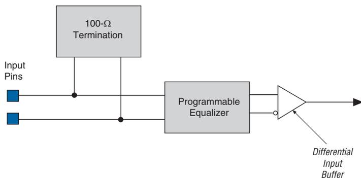
If a design uses external termination, the receiver must be externally terminated and biased to 0.85 V or 1.2 V. Figure 2-12 shows an example of an external termination and biasing circuit.
