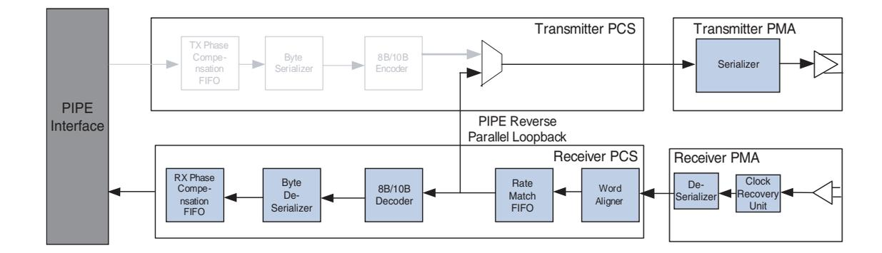
You can dynamically put the PCI Express (PIPE) mode transceiver in reverse parallel loopback by controlling the `tx_detectrxloopback` port instantiated in the MegaWizard Plug-In Manager. A high on the `tx_detectrxloopback` port in P0 power state puts the transceiver in reverse parallel loopback. A high on the `tx_detectrxloopback` port in any other power state does not put the transceiver in reverse parallel loopback.
