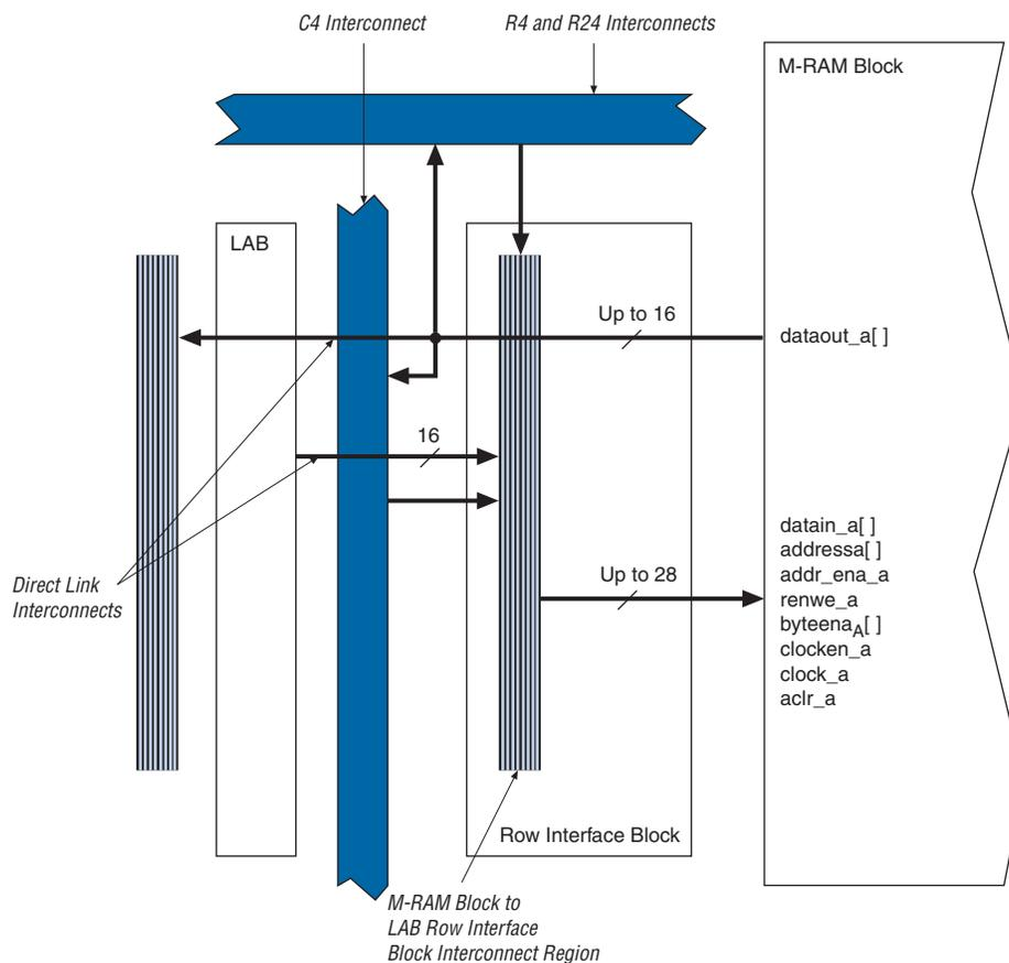
Table 2-12 lists the input and output data signal connections along with the address and control signal input connections to the row unit interfaces (L0 to L5 and R0 to R5).
