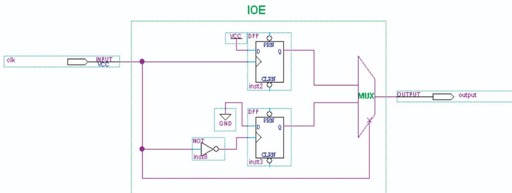
When an FPGA PLL generates the internal clock, the PLL output clocks the IOE block. As the PLL only monitors the positive edge of the reference clock input and internally re-creates the output clock signal, any DCD present on the reference clock is filtered out. Therefore, the DCD for a DDIO output with PLL in the clock path is better than the DCD for a DDIO output without PLL in the clock path.
