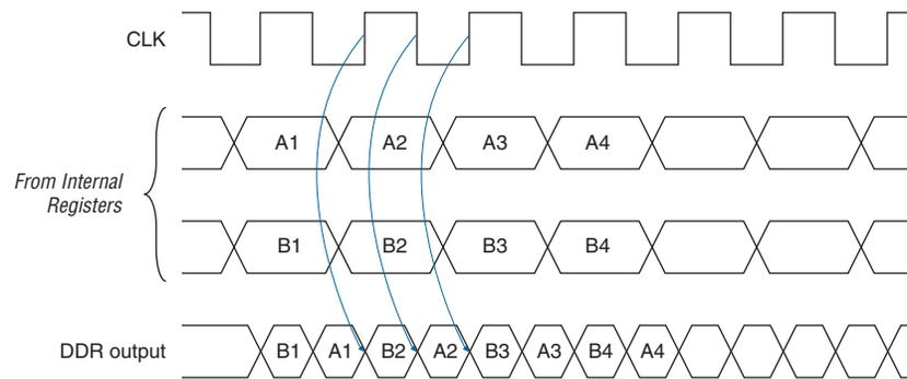
The Arria GX IOE operates in bidirectional DDR mode by combining the DDR input and DDR output configurations. The negative-edge-clocked OE register holds the OE signal inactive until the falling edge of the clock to meet DDR SDRAM timing requirements.
