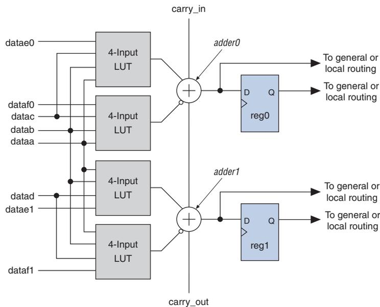
While operating in arithmetic mode, the ALM can support simultaneous use of the adder's carry output along with combinational logic outputs. In this operation, adder output is ignored. This usage of the adder with the combinational logic output provides resource savings of up to 50% for functions that can use this ability. An example of such functionality is a conditional operation, such as the one shown in Figure 2-35. The equation for this example is:
