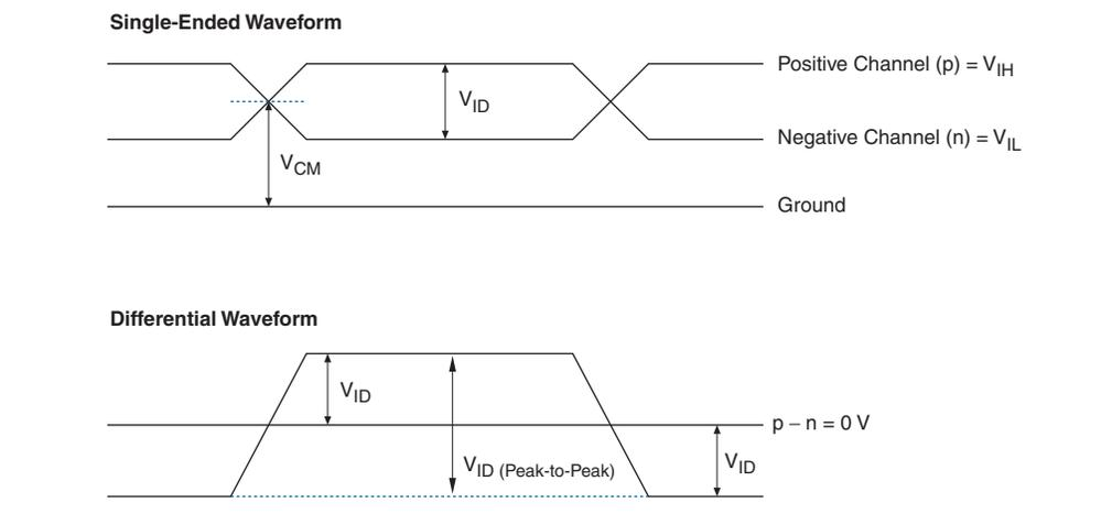
**Figure 4-6.** Transmitter Output Waveforms for Differential I/O Standards
