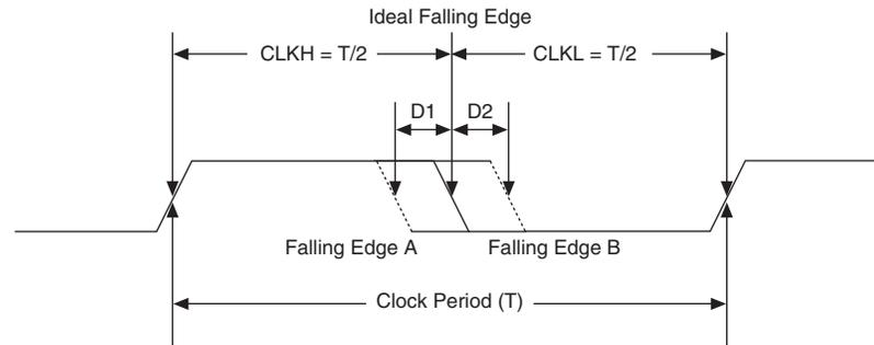
DCD expressed in absolute derivation, for example,  $D1$  or  $D2$  in Figure 4-10, is clock-period independent. DCD can also be expressed as a percentage, and the percentage number is clock-period dependent. DCD as a percentage is defined as:
