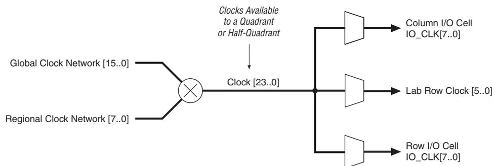
You can use the Quartus II software to control whether a clock input pin drives either a GCLK, RCLK, or dual-RCLK network. The Quartus II software automatically selects the clocking resources if not specified.
