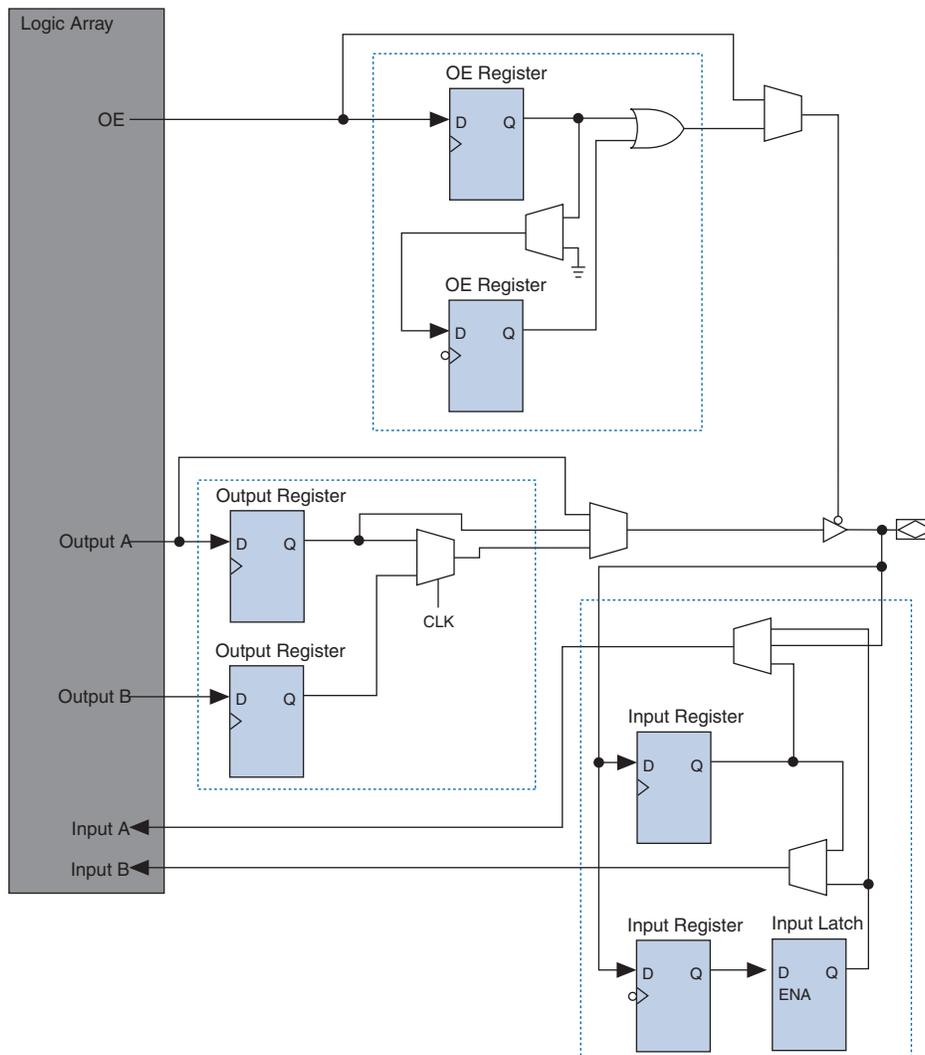
The IOEs are located in I/O blocks around the periphery of the Arria GX device. There are up to four IOEs per row I/O block and four IOEs per column I/O block. Row I/O blocks drive row, column, or direct link interconnects. Column I/O blocks drive column interconnects.
