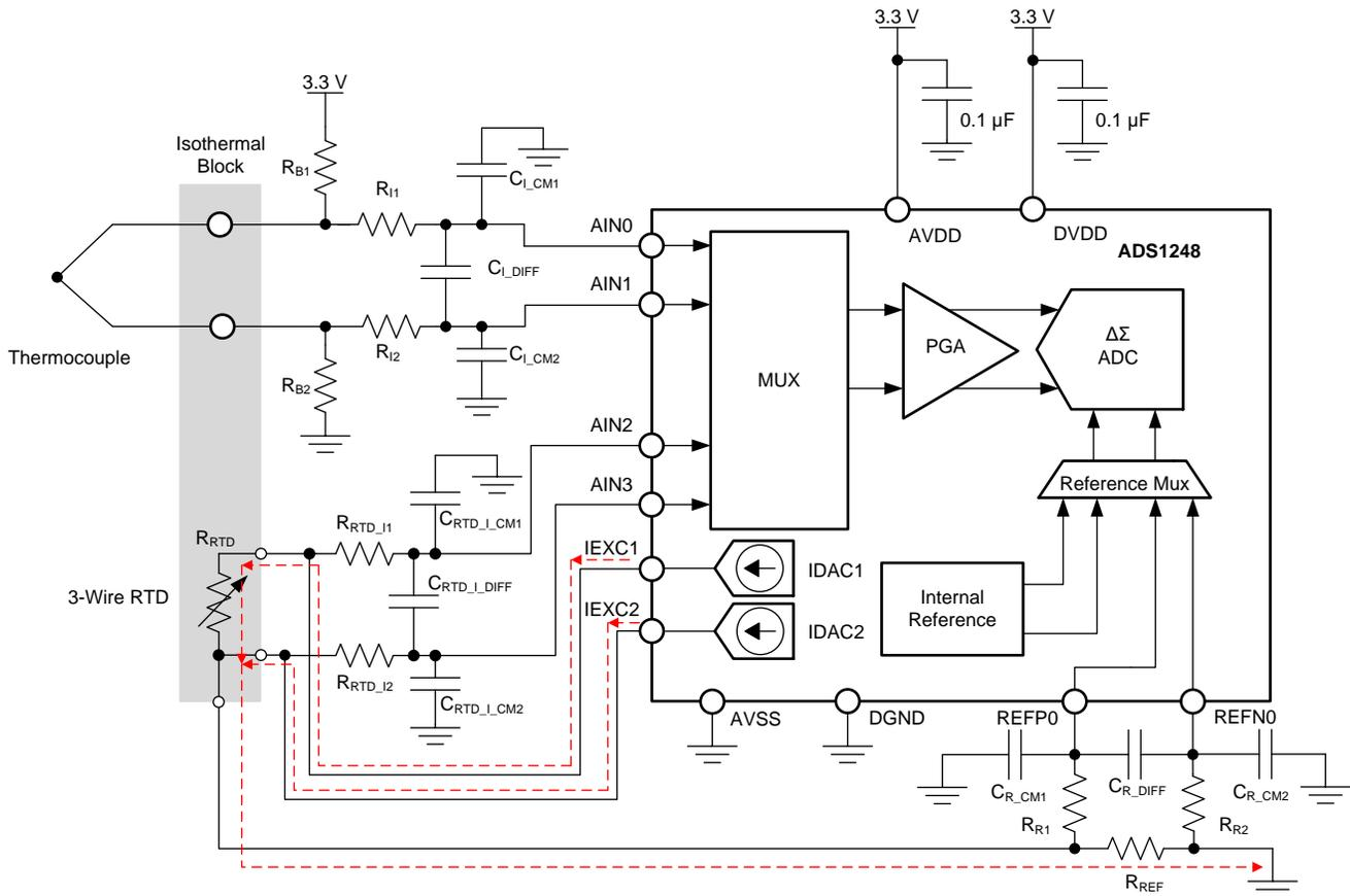
Figure 120. Thermocouple Measurement System Using the ADS1248
