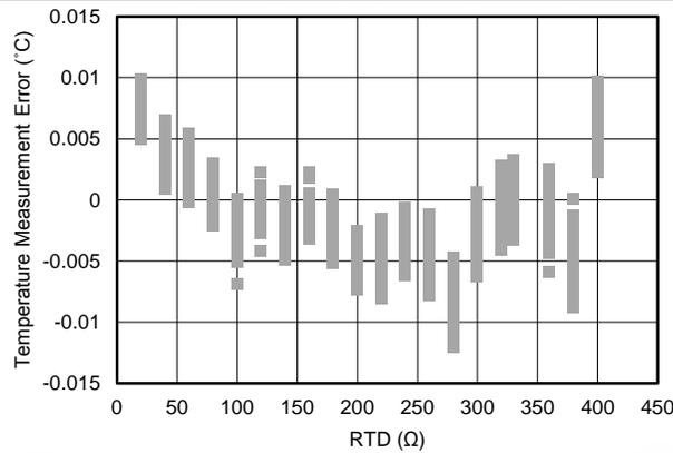
Figure 119. Calculated Temperature Error from Resistance Measurement Error
