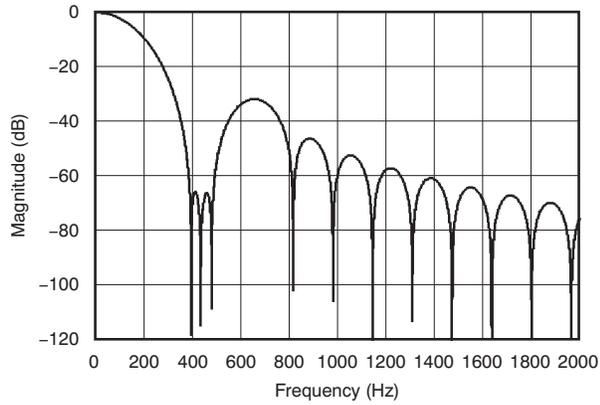
**Figure 63. Filter Profile with Data Rate = 160 SPS**
