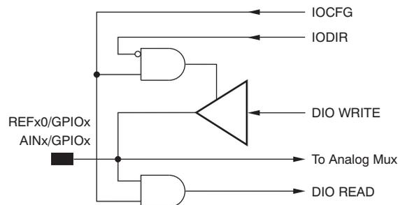
**Figure 69. Analog and Data Interface Pin**
