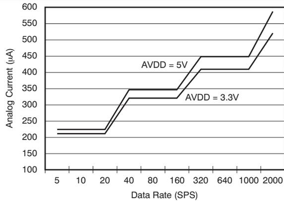
Figure 43. Analog Supply Current vs Data Rate
