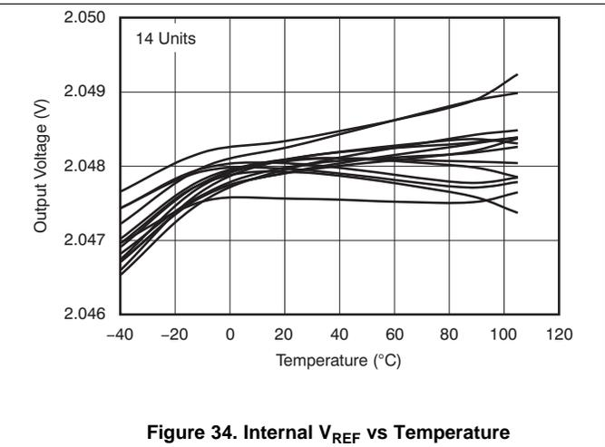
Figure 34. Internal  $V_{REF}$  vs Temperature
