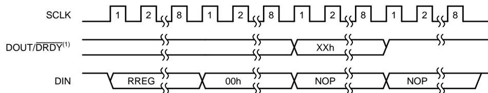
(1) DRDY MODE bit enabled,  $\overline{CS}$  tied low.
