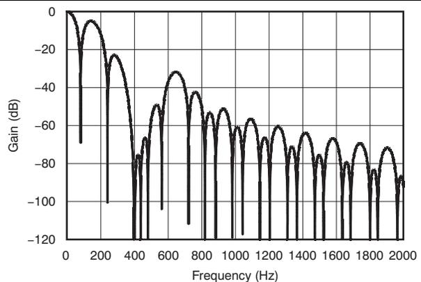
Figure 62. Filter Profile with Data Rate = 80 SPS
