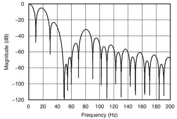
Figure 58. Filter Profile with Data Rate = 10 SPS
