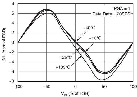
Figure 5. Integral Nonlinearity vs Input Signal
