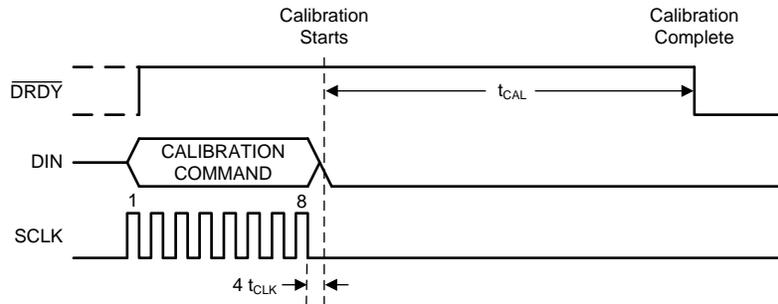
**Figure 86. Calibration Command**
