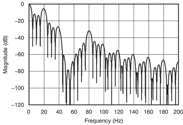
Figure 57. Filter Profile with Data Rate = 5 SPS
