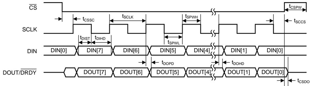
Figure 1. Serial Interface Timing, DRDY MODE Bit = 0
