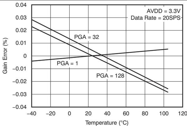
**Figure 21. Gain Error vs Temperature**
