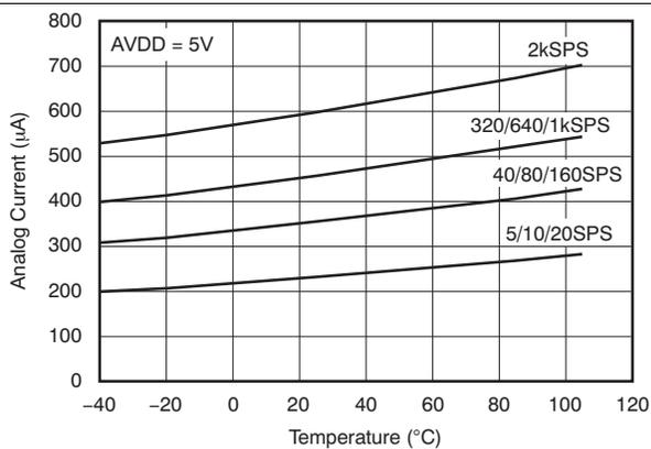
Figure 45. Analog Supply Current vs Temperature
