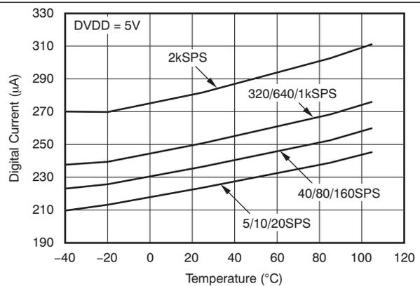
Figure 46. Digital Supply Current vs Temperature
