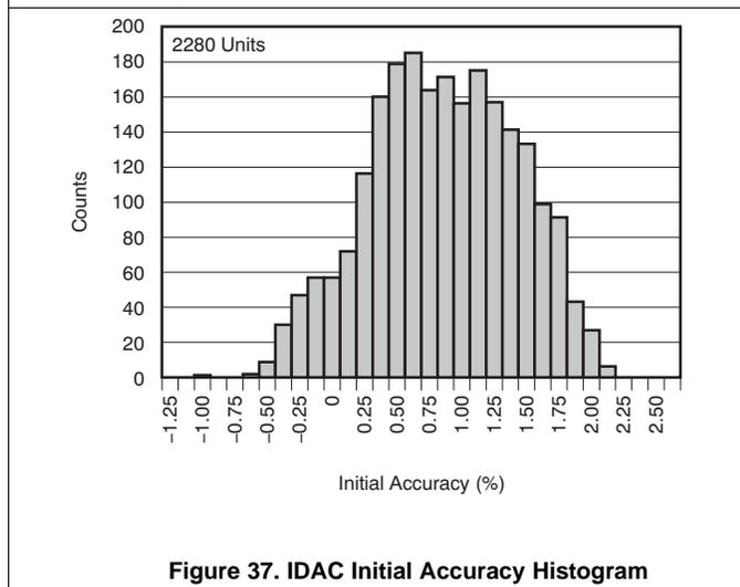
Figure 37. IDAC Initial Accuracy Histogram
