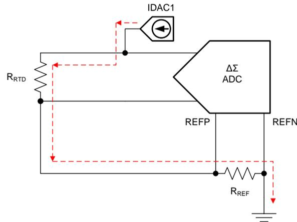
Figure 115. Example of a Ratiometric RTD Measurement
