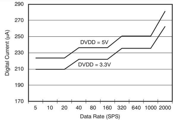
Figure 44. Digital Supply Current vs Data Rate
