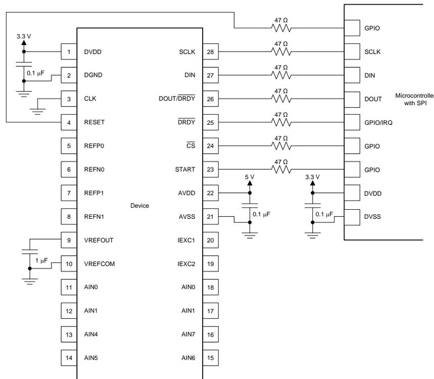
**Figure 110. Serial Interface Connections**
