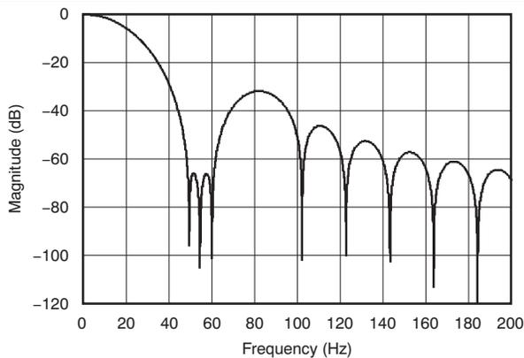
Figure 59. Filter Profile with Data Rate = 20 SPS
