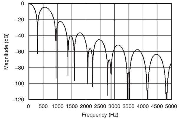
**Figure 64. Filter Profile with Data Rate = 320 SPS**
