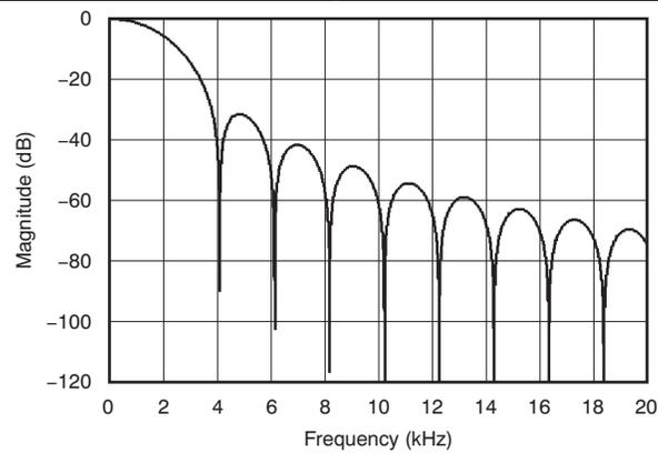
**Figure 67. Filter Profile with Data Rate = 2 kSPS**
