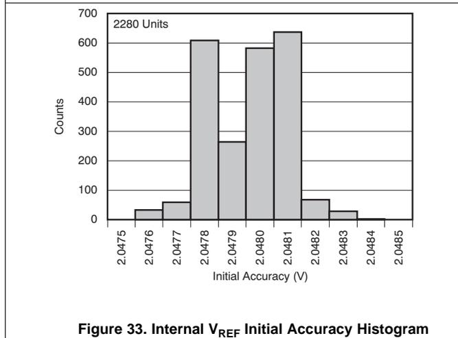
Figure 33. Internal  $V_{REF}$  Initial Accuracy Histogram
