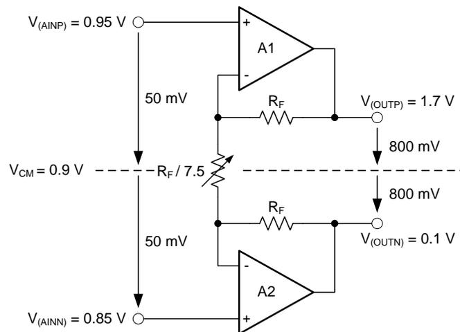
**Figure 54. Example where  $V_{CM}$  is at Lowest Limit**
