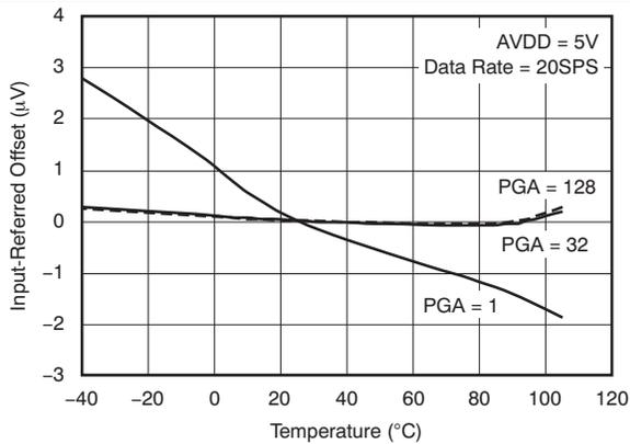
Figure 9. Offset vs Temperature
