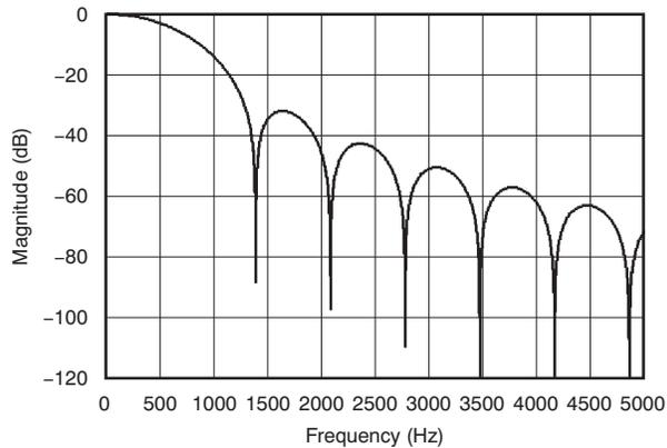
**Figure 65. Filter Profile with Data Rate = 640 SPS**
