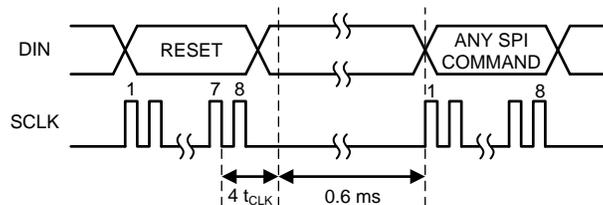
**Figure 80. SPI Communication after an SPI Reset**
