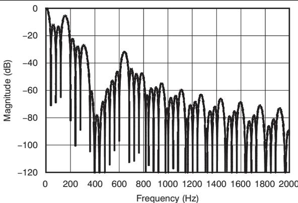
Figure 61. Filter Profile with Data Rate = 40 SPS
