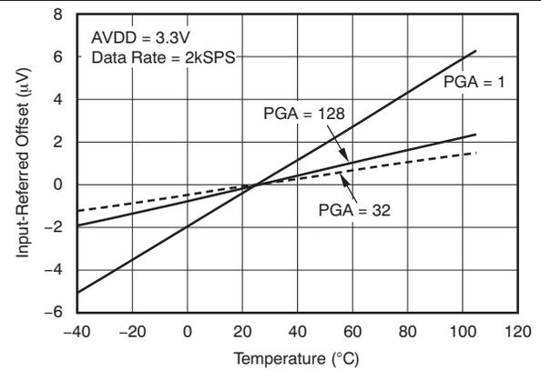
Figure 16. Offset vs Temperature
