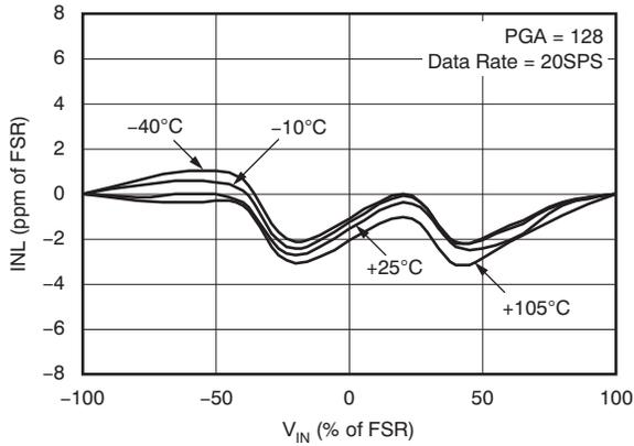
Figure 7. Integral Nonlinearity vs Input Signal
