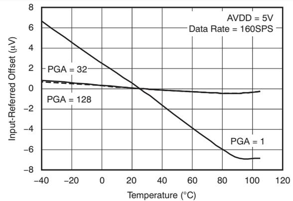
Figure 10. Offset vs Temperature
