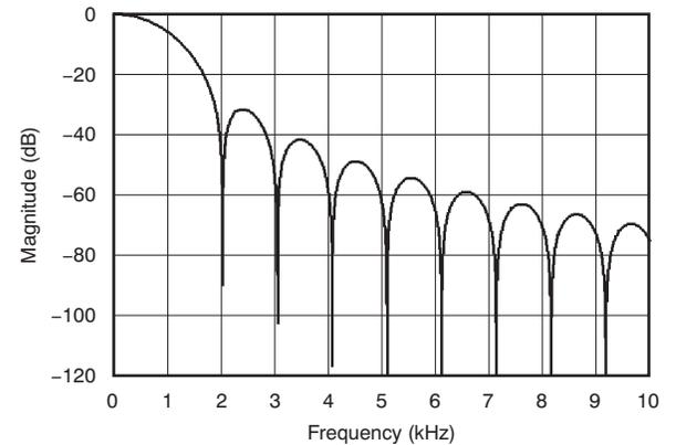
**Figure 66. Filter Profile with Data Rate = 1 kSPS**
