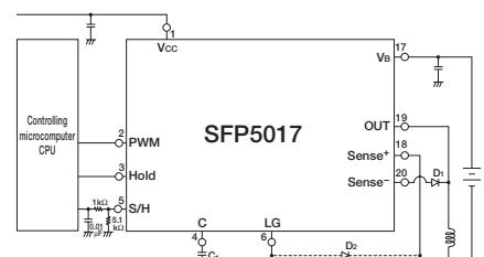
\* Use a Schottky Di for D2 when the Sense+ terminal is lower than the abs. max. rated voltage (-0.8V)
