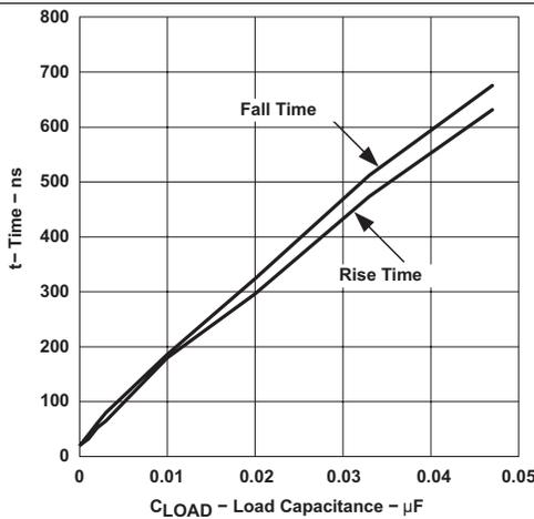
Figure 2. Gate Drive Timing vs Load Capacitance
