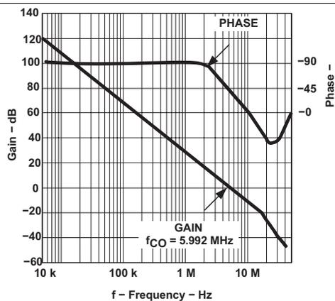
Figure 6. Current Amplifier Gain vs Frequency
