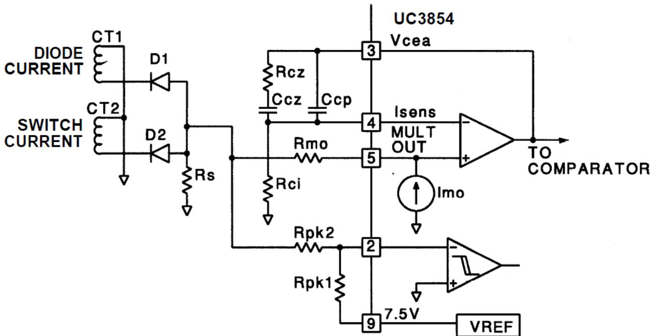
Figure 10. Current Transformers Used With Negative Output
