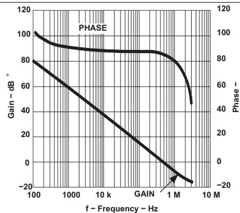
Figure 7. Voltage Amplifier Gain vs Frequency
