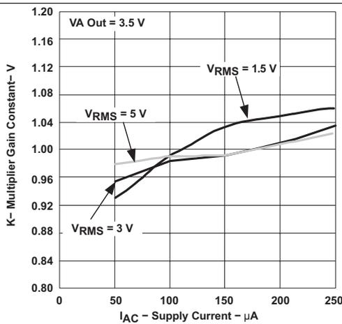
Figure 4. Multiplier Gain Constant vs Supply Current
