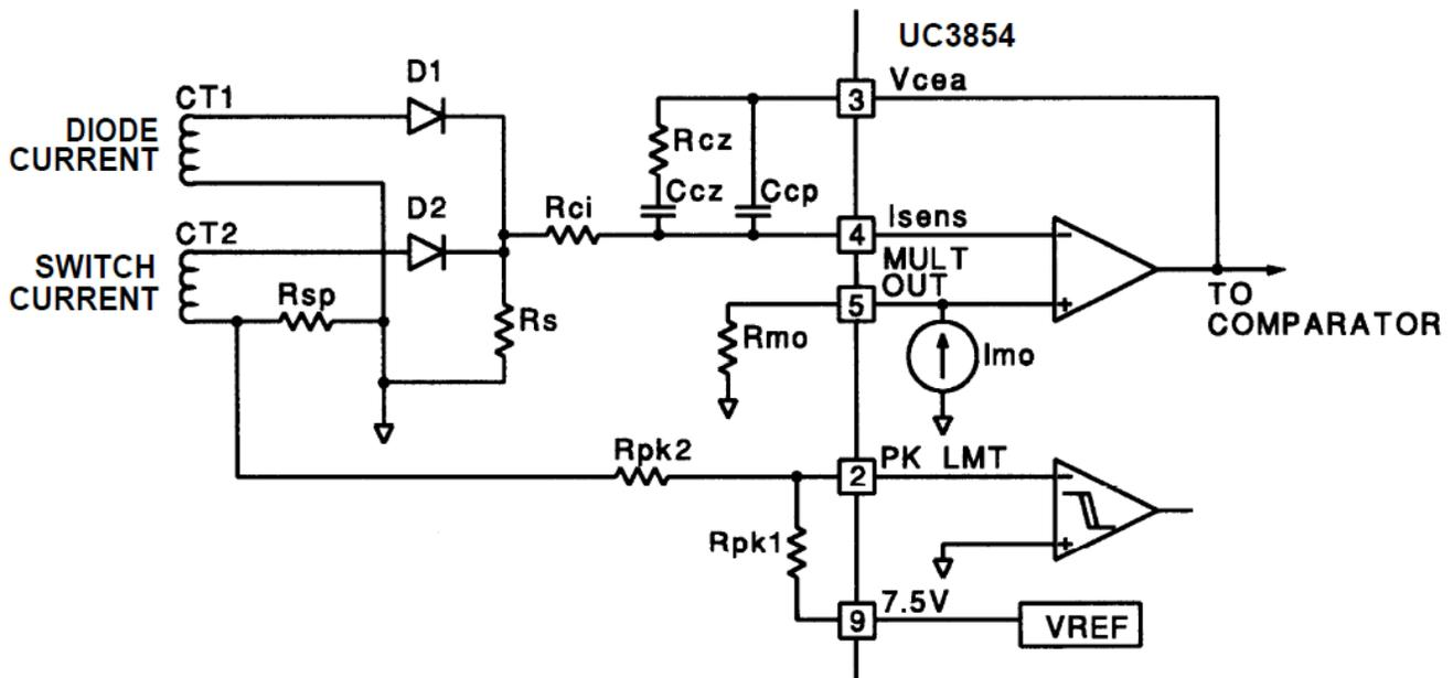
Figure 11. Current Transformers Used With Positive Output
