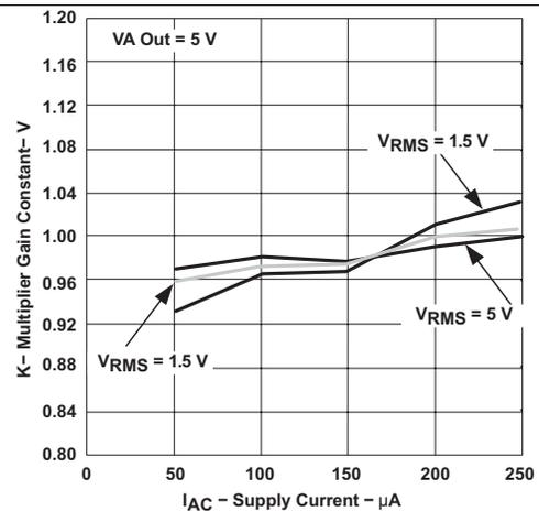
Figure 5. Multiplier Gain Constant vs Supply Current
