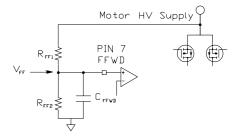
Fig. 7 Feedforward Connection Diagram
