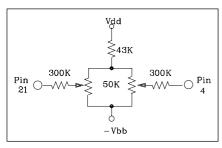
Fig. 10b Input Offset Adjust Circuit
