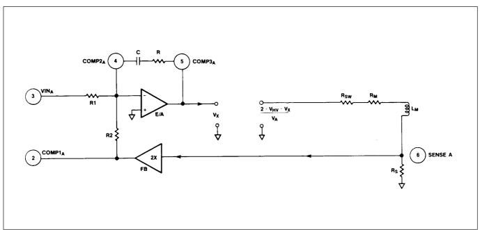
Fig. 11a Loop Compensation Block Diagram
