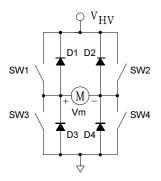
Fig. 8 Simplified H-Bridge Diagram
