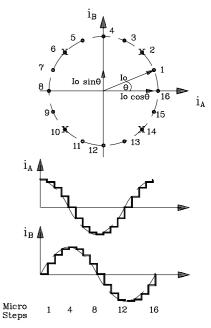
Fig. 2 Four Microstep per Step Drive Waveforms
