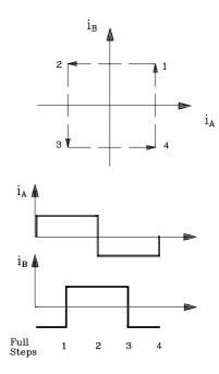
Fig. 1 Full Step Drive Waveforms
