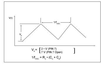
Fig. 6b: Oscillator Waveform Diagram
