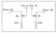
Fig. 10c Gain Adjust Circuit
