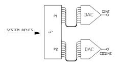
Fig. 5 Microprocessor Based Referenced Waveform Generator
