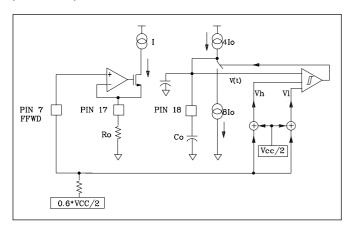
Fig. 6a: Oscillator Block Diagram
