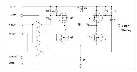
Fig. 9 AC Coupled H-Bridge Diagram
