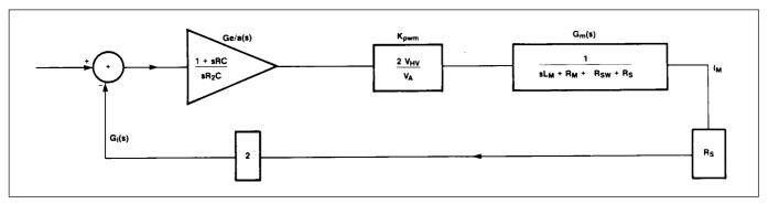
Fig. 11b Simplified laplace transform for stability analysis
